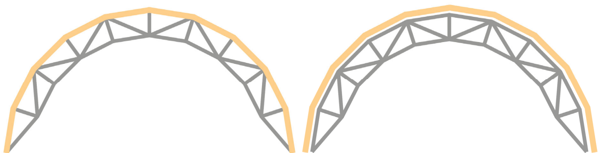
Figure 88: Redefinition interaction between trusses and main structure
