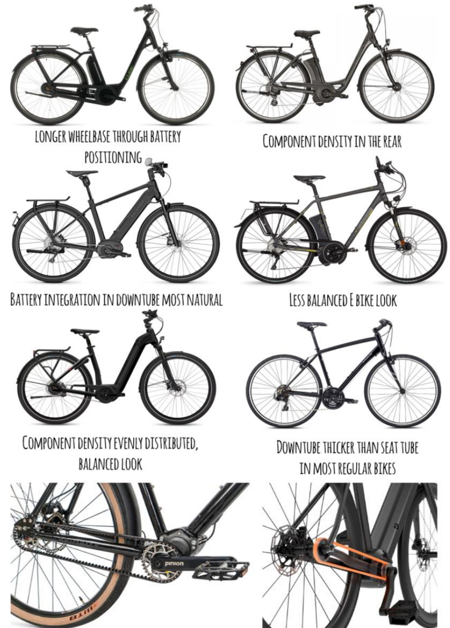
Figure 10: E-bike aesthetics based on battery position and an openness of the belt without a chainguard.
