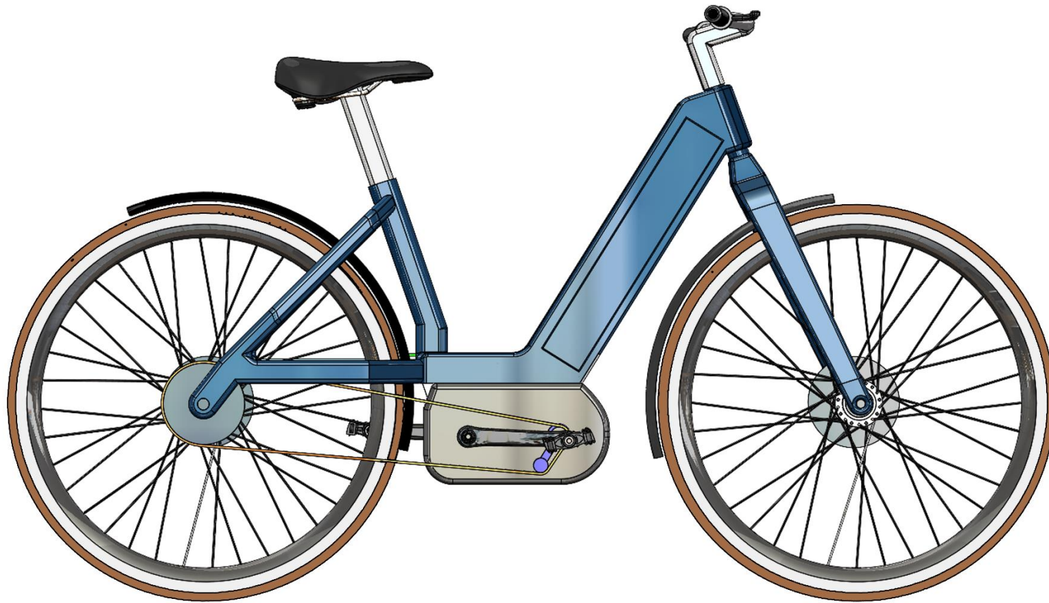
Figure 41: The final E-bike design revolved around the modular system.
