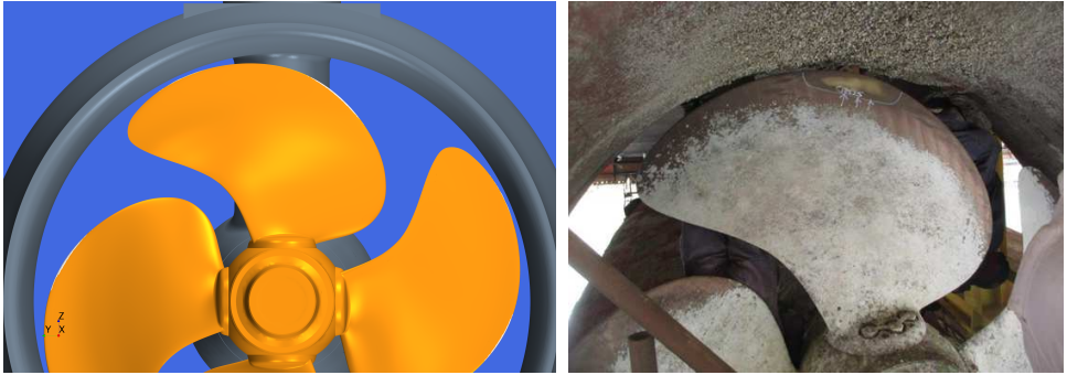
Figure 5.34: Representation of the vapor volume on the blades of the second re-design, in dynamic positioning (left), and the actual damage on the real blade (right)
