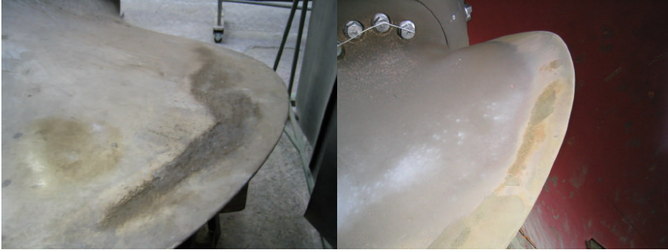
Figure 6.3: Actual erosion on the blades for Design 1 (left) and Design 2 (right). The exact period over which each propeller design had been operated to get the depicted erosion damage is unknown.
