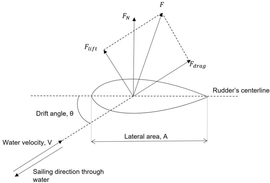
Figure 3.5: Top view of rudder with corresponding forces when the rudder is not aligned with the sailing direction
