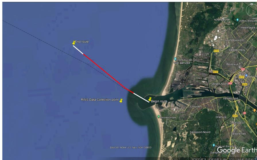
Figure 4.6: IJmuiden sea access, RWS measuring pole and the Volvox Olympia sailing route. The white segment of the path indicates the acceleration/deceleration part, the red segment of the path indicates the free sailing part. (Source: Google Earth Pro. [Screenshots]. Retrieved from <https://www.google.com/earth/versions/earth-pro>, 06-05-2023)
