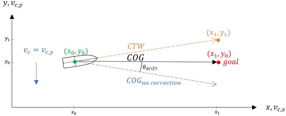
Figure 3.11: Scenario 2: sailing in x-direction, perpendicular current
