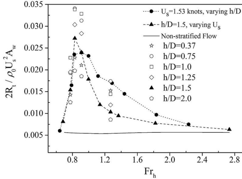
Figure 3.9: Dimensionless total resistance for an increasing densimetric Froude number and different ratios of draught to total water depth ( $h/D$ ) (Esmailpour et al., 2018)
