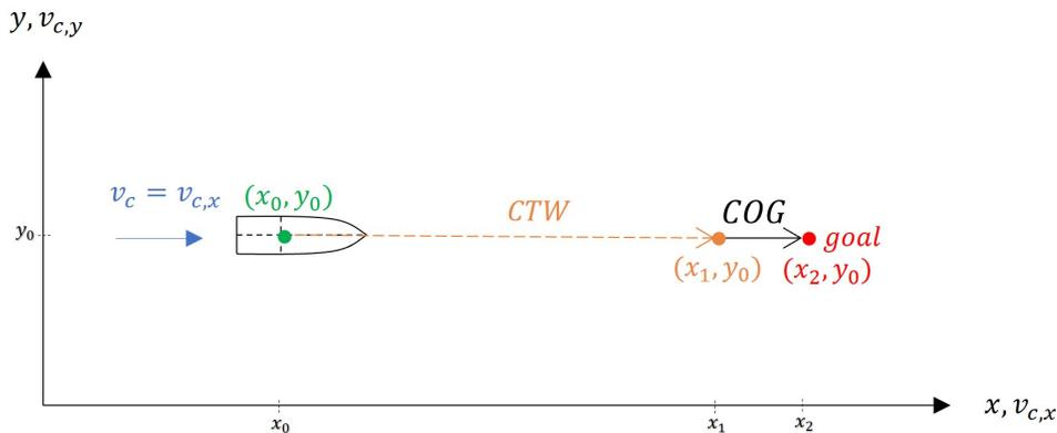
Figure 3.10: Scenario 1: sailing in x-direction, parallel current
