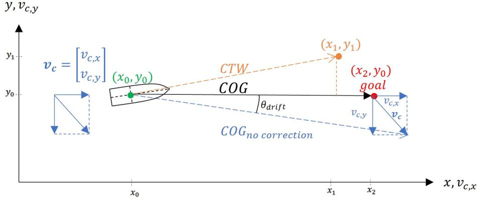
Figure 3.12: Scenario 3: sailing in x-direction, current has a perpendicular and parallel component
