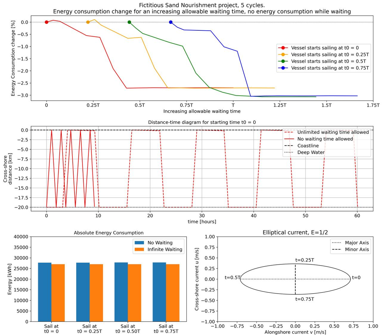
Figure 4.13: Results for sailing 5 cycles. Relative energy consumption change compared to no allowable waiting time for four different starting times ( $t_0 = 0$  (top), time-distance diagram for starting time  $t_0 = 0$  (middle), absolute energy consumption change (bottom left) and ellipticity  $E = 1/2$  (bottom right).
