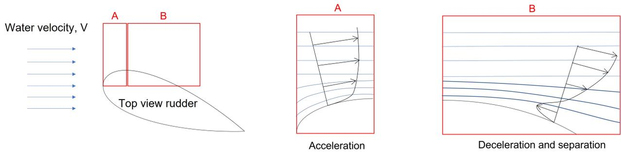
Figure 3.4: Top view of rudder, highlighting the acceleration zone (A) and decelerating or separation zone (B)
