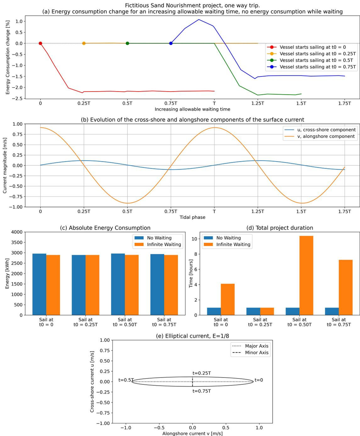
Figure D.2: Results for sailing a one way trip. Relative energy consumption change compared to no allowable waiting time for four different starting times (a), cross-shore and alongshore components at  $x = -20\text{km}$  (b), absolute energy consumption change (c) and total project duration (d). Ellipticity  $E = 1/8$  (e).
