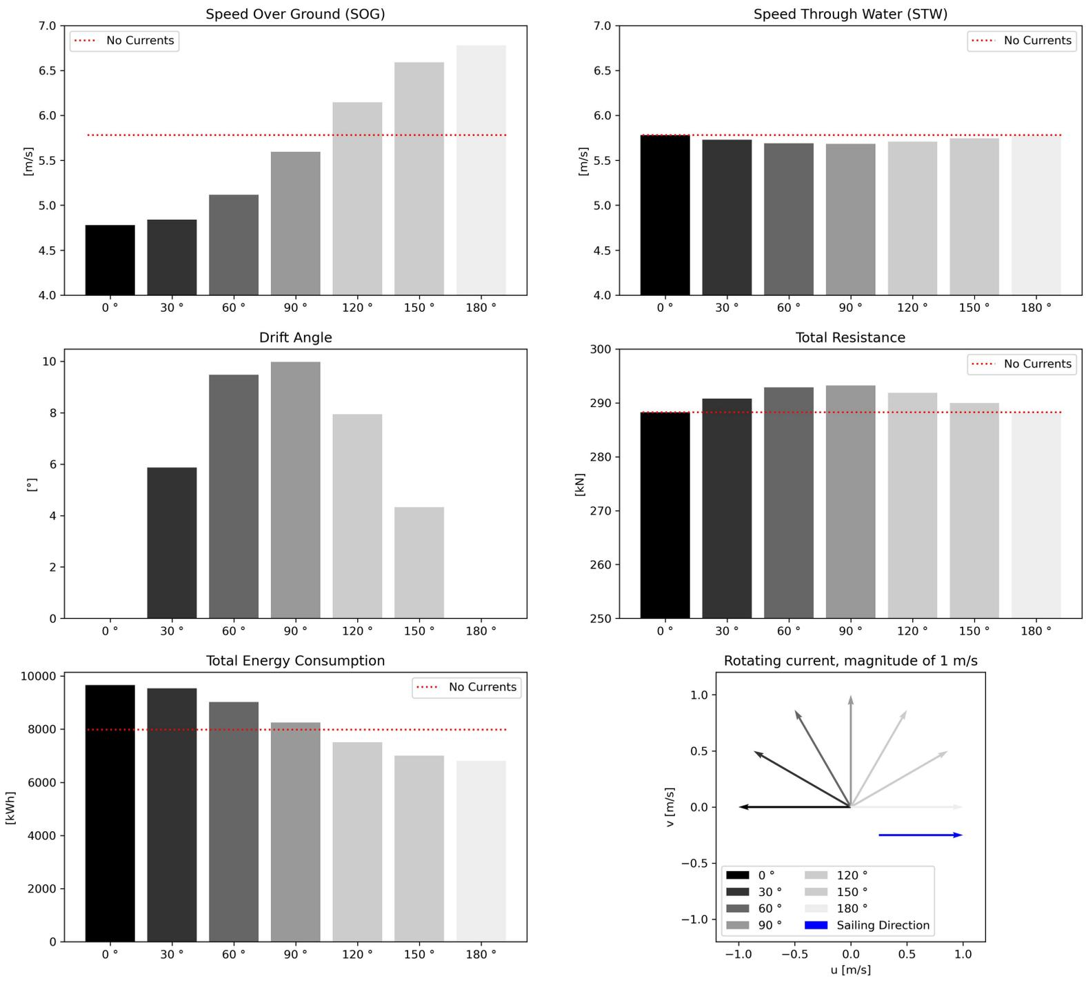
Figure 4.3: Test case 5: varying space- and time independent currents
