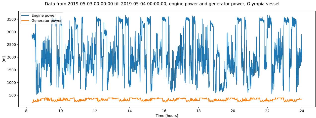
Figure 4.14: Engine power and generator power of the Volvox Olympia for a time period of 24 hours during the IJgeul sea access project.
