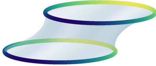
Figure 2.1: The minimal surface between two circles which are close to each other is a so called catenoid. Note that the boundary is made up of two unconnected curves.
