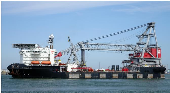
Figure A.2: The Oleg Strashnov vessel, fitted with a single 5000 mton capacity crane.
