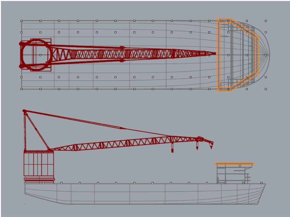
Figure 3.4: Monohull general arrangement drawings of the main deck.
