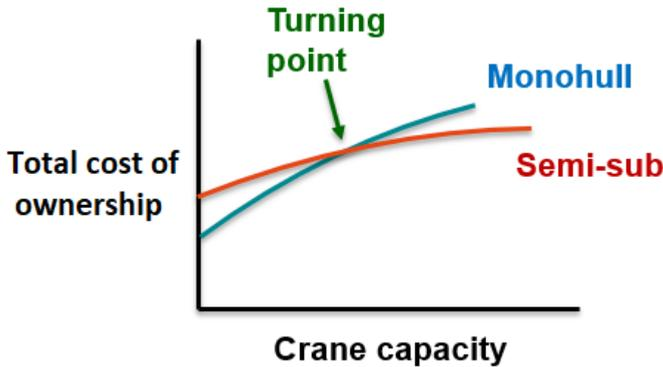
Figure 2.3: Schematic impression of the cost (Operational and capital) that depends on the crane capacity of the vessel.
