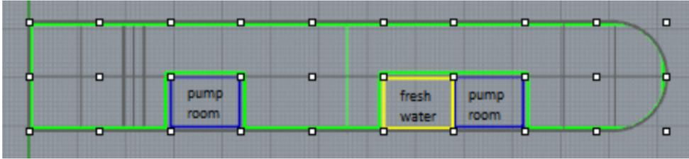
Figure 4.5: Semi-sub general arrangement of the floater. All space is used for ballast tanks unless otherwise indicated for the pump rooms and fresh water tank.
