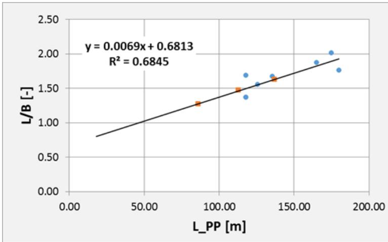
Figure E.10: Semi-submersible: Length-width ratio as function of the vessel length.
