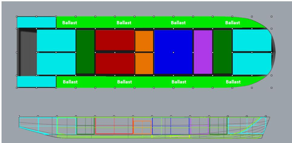
Figure 3.6: Monohull general arrangement of the internal components, including the ballast tanks.
