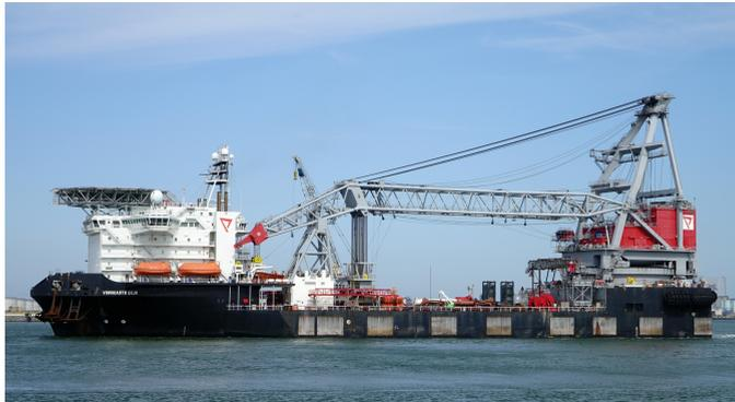
Figure 1.1: The Oleg Strashnov vessel, fitted with a single 5000 mton capacity crane.
