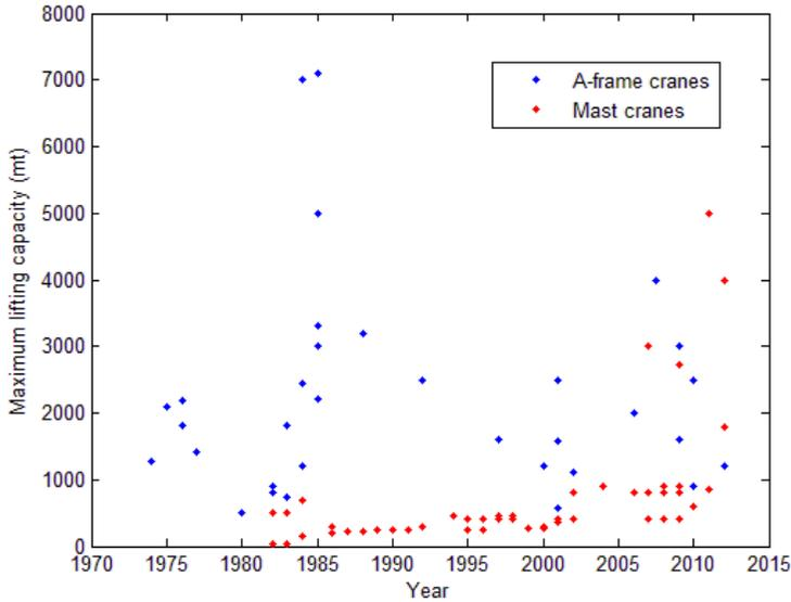
Figure F.3: Number of mast and A-frame cranes with their crane capacities over the years.
