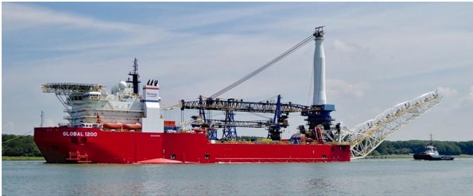
Figure A.3: The Global 1200 vessel, capable of heavy lift and pipelay operations. The crane has a 1200 mton capacity.
