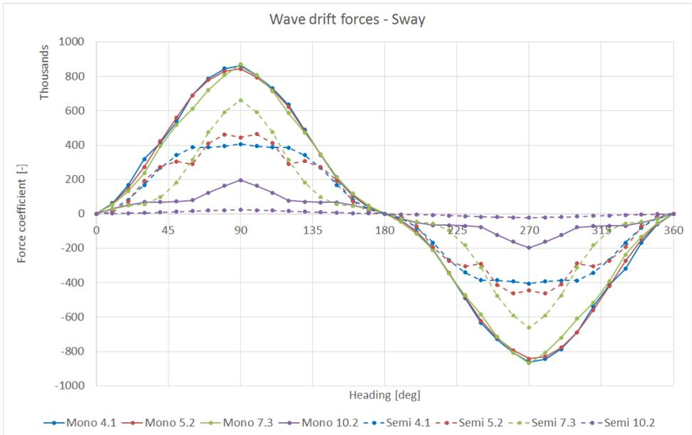
Figure 8.6: Wave drift sway forces for both vessel types for a selection of wave periods.
