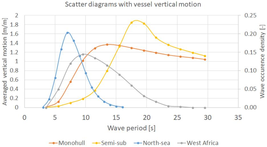
Figure 7.3: The north-sea and West africa wave scatter plot (blue and grey lines), together with an averaged vertical motion plot for both 6000 mt vessels.
