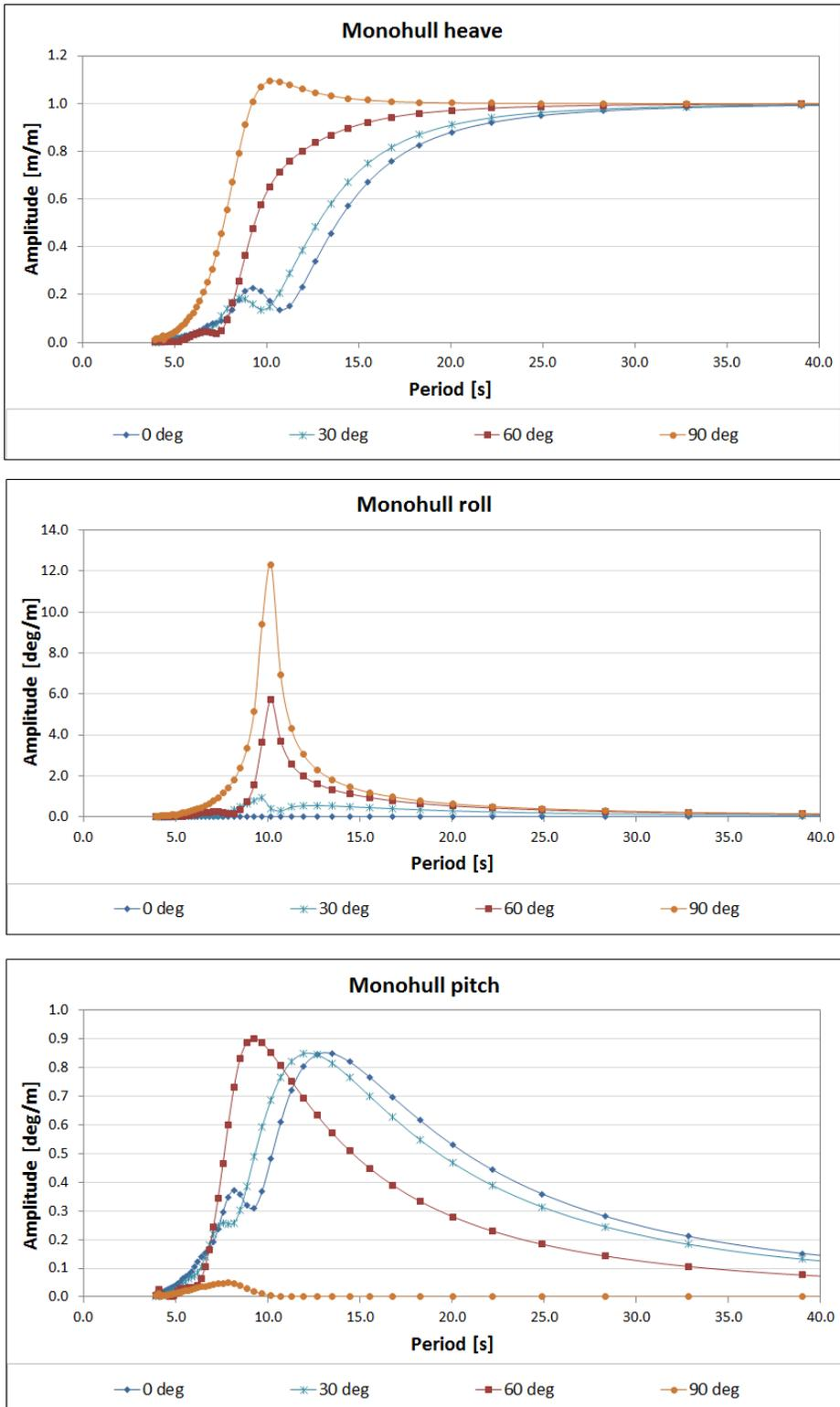
Figure 7.1: Monohull RAOs for heave, pitch and roll in the North-sea.
