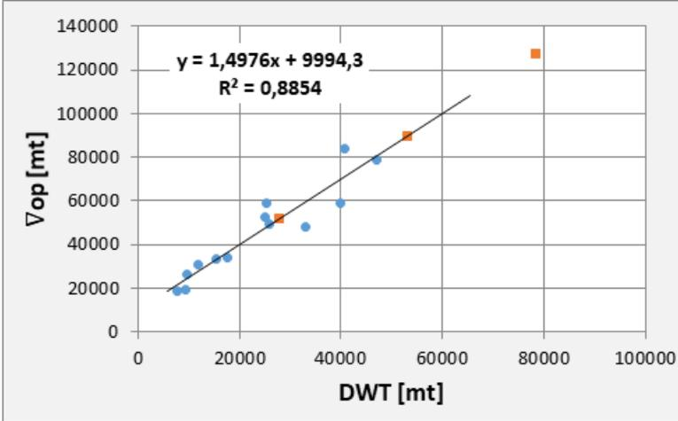
Figure E.3: Monohull: relation between the operational displacement ( $\nabla_{op}$ ) and deadweight tonnage ( $DWT$ ).
