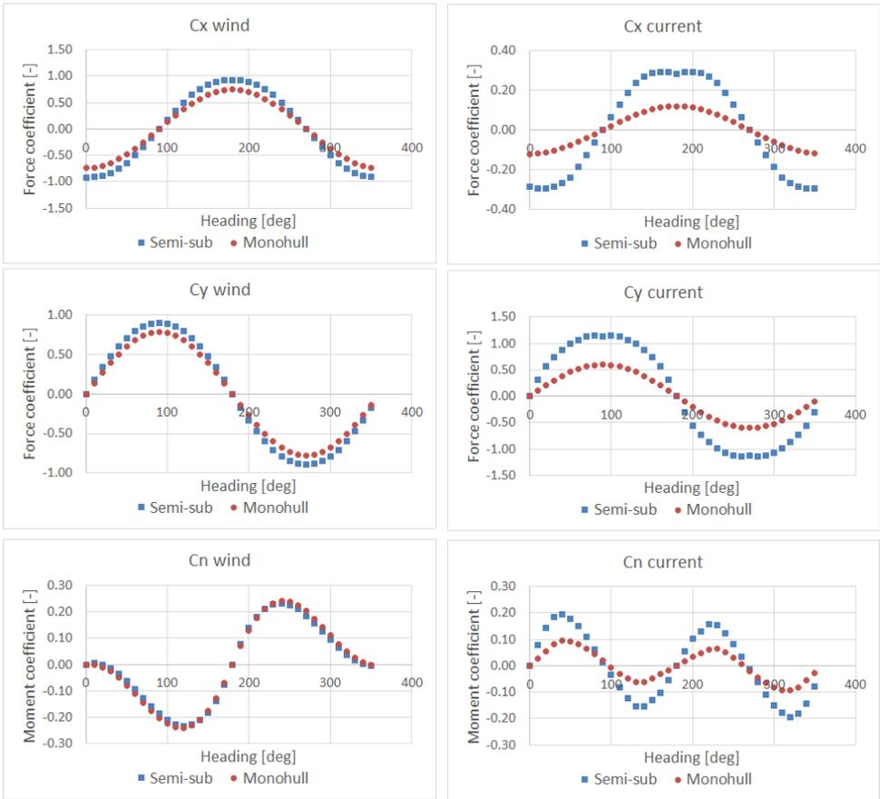
Figure 8.4: Wind and current force/moment coefficients for the monohull and semi-sub 6000mt design.
