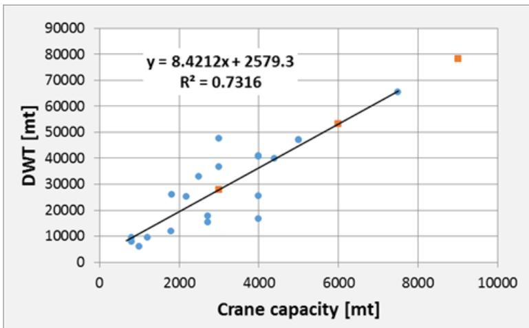
Figure E.2: Monohull: relation between the crane capacity ( $Q$ ) and Deadweight tonnage ( $DWT$ ) of the vessel.
