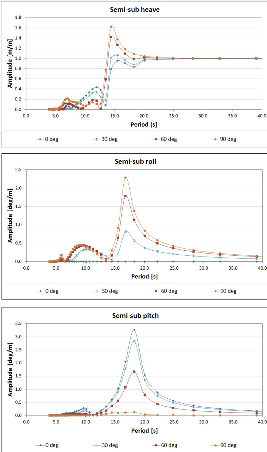
Figure 7.2: Semi-sub RAOs for heave, pitch and roll in the North-sea.
