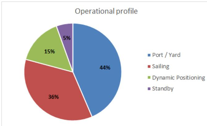
Figure 2.1: General heavy lift vessel operational profile.
