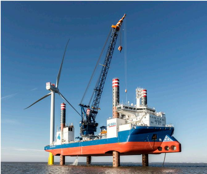
Figure A.4: A jack-up vessel, capable of lifting itself above the water surface.
