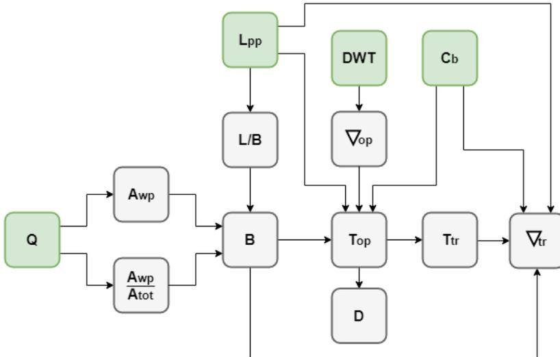
Figure 4.1: Main parameters selection flow for the semi-sub designs. Green boxes mean it is either an input or chosen parameter.
