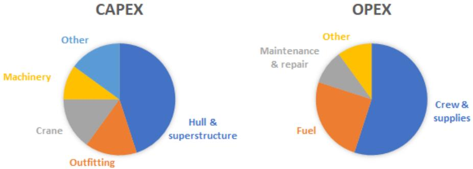
Figure 2.2: Estimated capital (left chart) and operational expenditures (right chart) for a heavy lift crane vessel. (citations)
