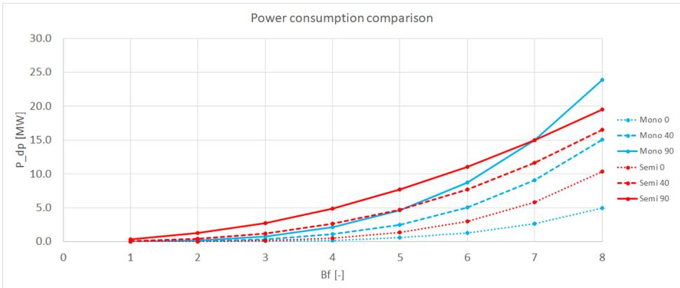
Figure 8.8: Required DP power for a range of environmental conditions for both vessel types, for a few headings.
