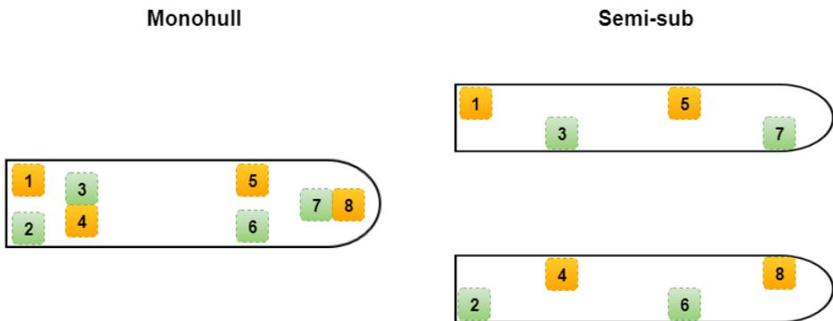
Figure 8.2: Monohull (left) and Semi-submersible (right) thruster division over the switchboards.
