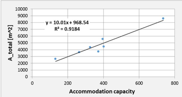
Figure E.19: The accommodation floor area as function of the accommodation capacity.
