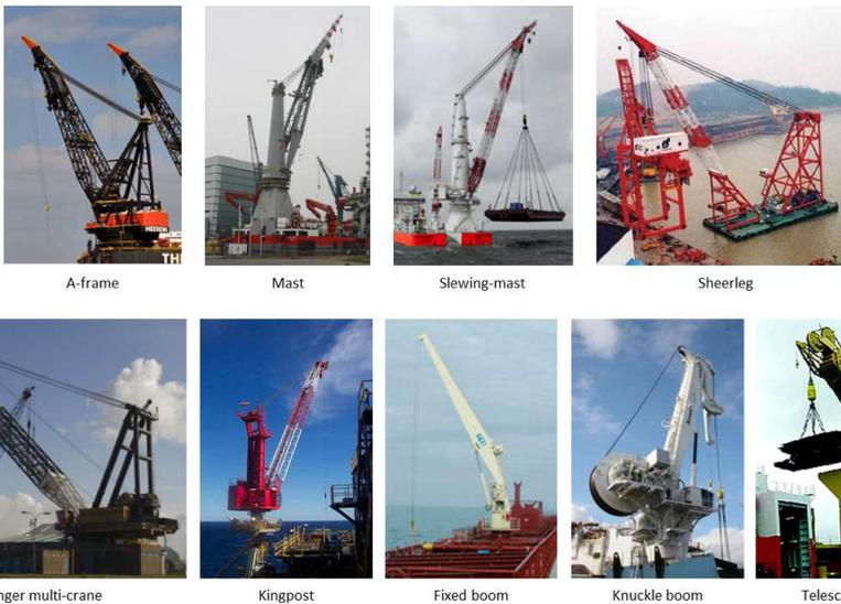
Figure F.1: The different types of cranes that can be used on-board ships. [17]
