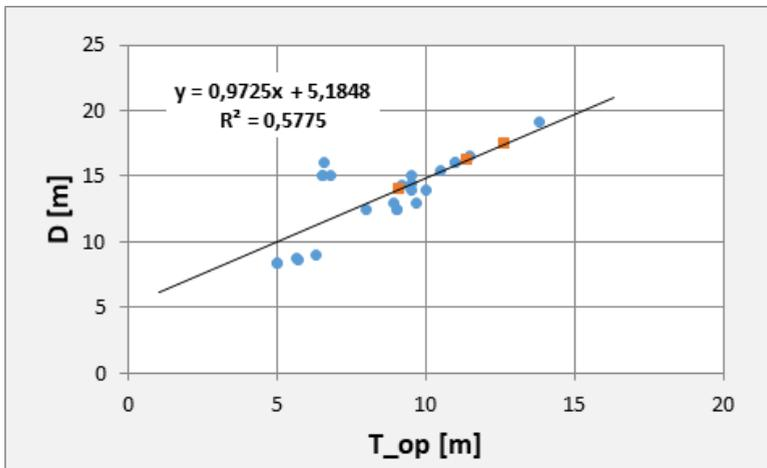
Figure E.5: Monohull: relation between the operational draft ( $T_{op}$ ) and depth ( $D$ ).
