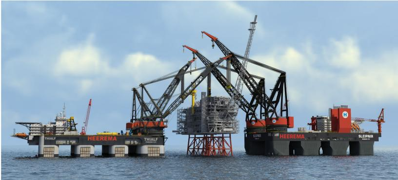
Figure 1.2: Two multihull semi-submersible ships carrying out an operation. On the left the Thialf with a combined crane capacity of 14200 tonnes, and on the right the Sleipnir, which is still under construction, with a combined crane capacity of 20000 tonnes
