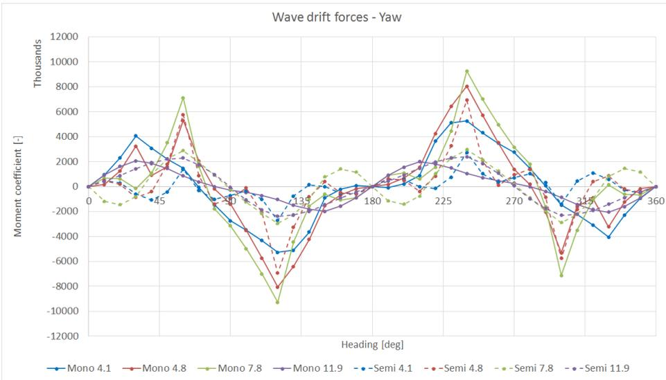
Figure 8.7: Wave drift yaw forces for both vessel types for a selection of wave periods.
