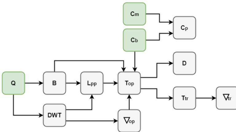
Figure 3.1: Main parameters selection flow for the monohull designs. Green boxes mean it is either an input or chosen parameter.
