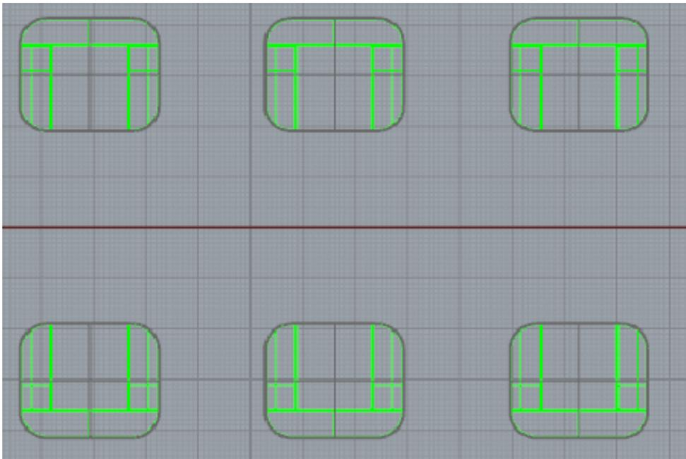
Figure 4.6: Semi-sub general arrangement of the columns. There are three ballast tanks fitted per columns. The rest of the space is reserved for other items such as thruster rooms and chain lockers.
