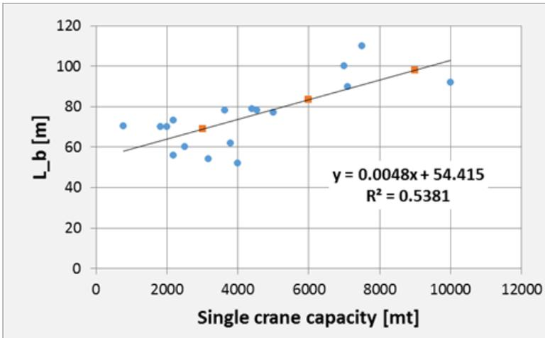
Figure E.16: Relation between the main boom length and single crane capacity.
