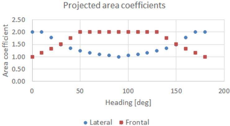
Figure 8.3: Projected area coefficients for the floater.
