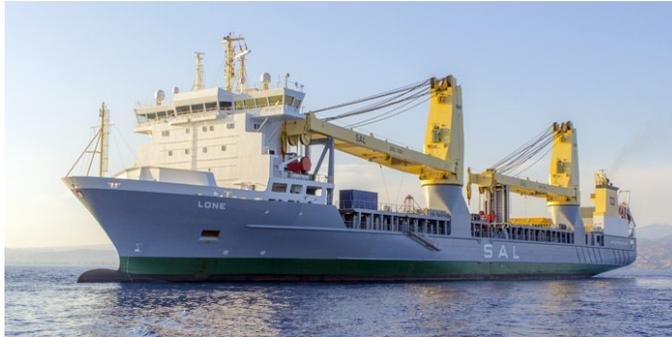
Figure A.1: The SAL type 176 vessel, fitted with 2 cranes of 700 mton capacity.
