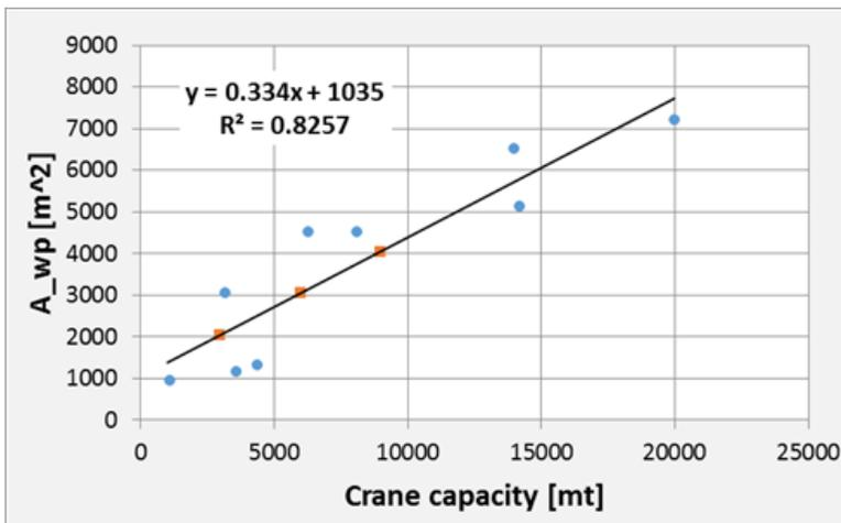
Figure E.8: Semi-submersible: Waterplane area as function of the crane capacity.
