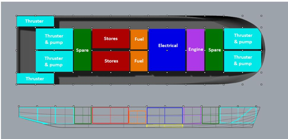
Figure 3.5: Monohull general arrangement of the internal components, except the ballast tanks. All items are separately indicated. The fresh water tanks can be seen in the bottom picture below the other items.
