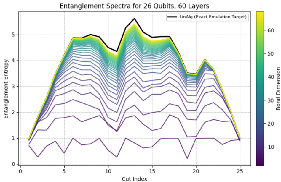
Figure 5.21: Evolution of the von Neumann entanglement distributions across natural cuts for a 26-qubit, 60-layer circuit as the MPS bond dimension increases. Each colored line corresponds to a different bond dimension, while the black line indicates the exact entanglement distribution calculated with the LinAlg emulator.
