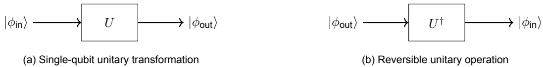
Figure 2.2: Comparison of a standard unitary transformation (left) with its corresponding reversible operation (right).
