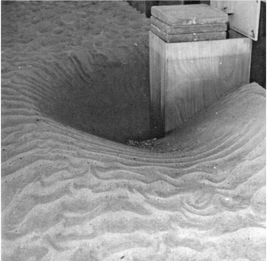
Scour in a horizontal constriction (photo Deltares)
