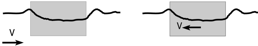
Figure 9-1 Flow around fixed object versus moving object in stagnant water
