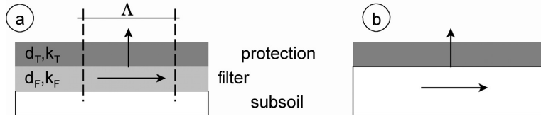
Figure 8-4 Definition leakage length
