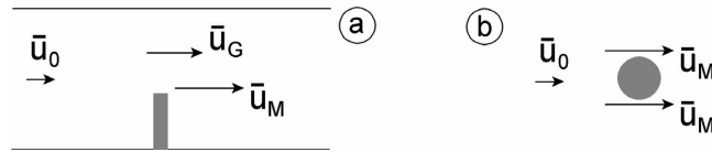
Figure 3-16 Definition of velocities in relation to K_v
