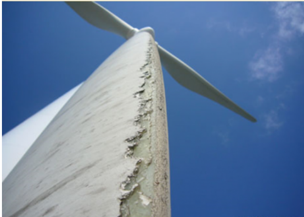
Figure 1.1: Leading-edge erosion damage on a wind turbine blade; photography reproduced from Telene (2021).
