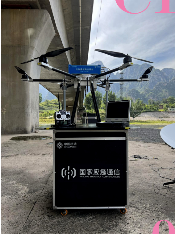
Fig. 3.13, Communication Base Station Drone-based emergency communication aerial base station
