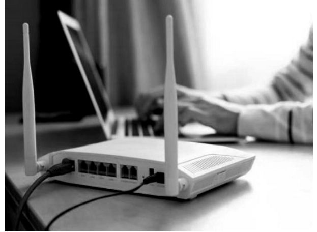
Fig. 3.50, Router Router directs data traffic by determining optimal paths, functioning as a key component of the Address Layer's routing system. Image source: https://192-168-1-1.com.cn/howto/2413.html
