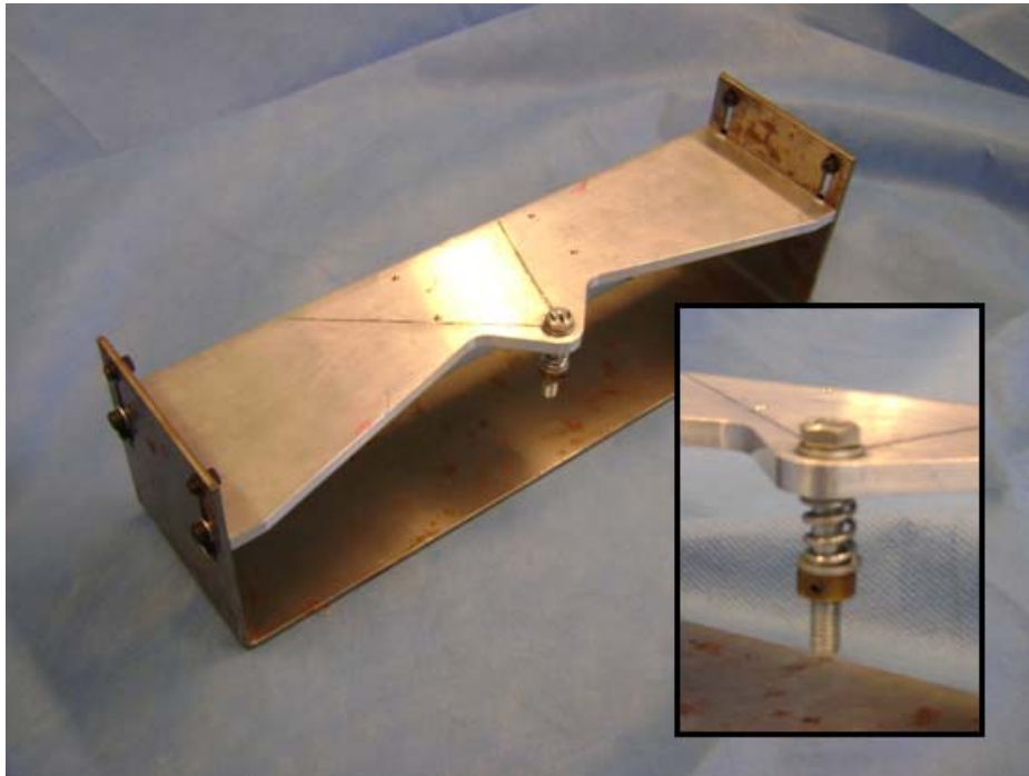
Figure 24: Task environment for a bolt and spanner task; a preloaded M6 bolt (designed by Wildenbeest, [Wildenbeest,2010]).
