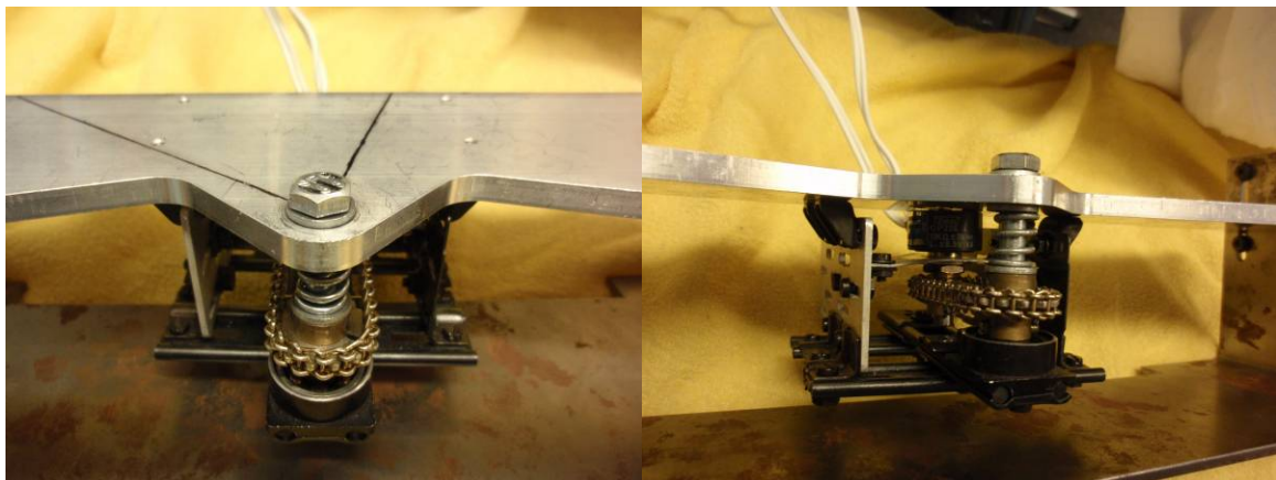
Figure 25: The bolt angle is measured using a potentiometer.
