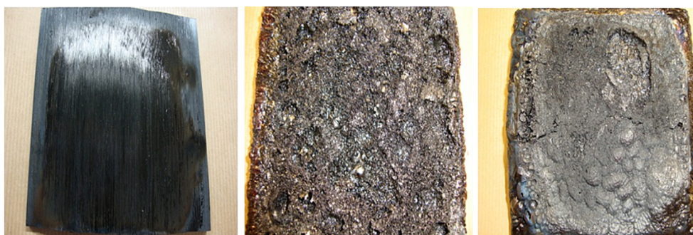
Figure 6. Digital photographs of three samples after fire testing (a) Uncoated composite (b) composite with unfilled coating (c) Composite with nano-filled coating.
