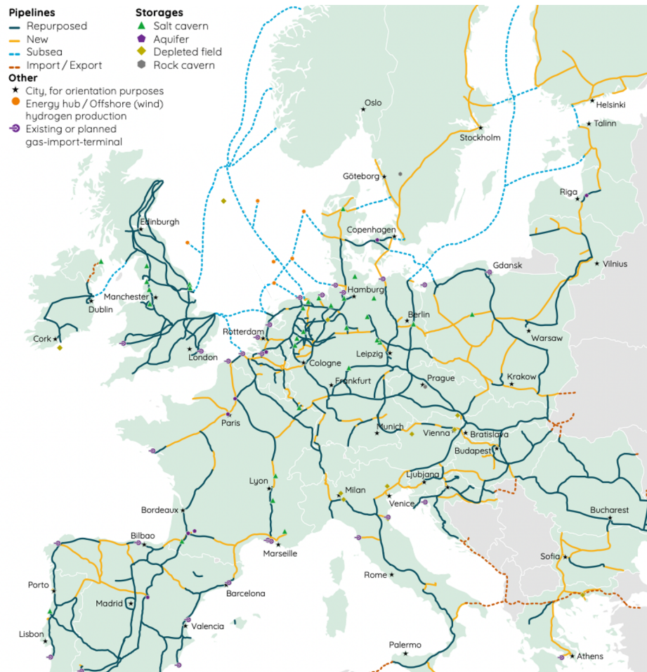
Figure 1.1: Expected mature hydrogen pipeline infrastructure in Europe by 2040. Adapted from [72].
