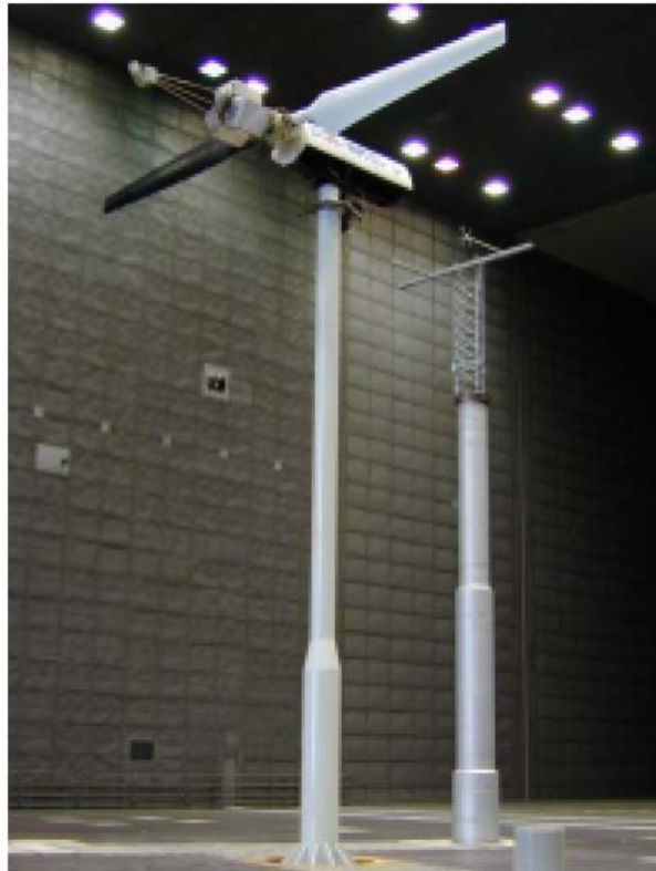
Figure 6.1 – The NREL Phase VI wind turbine in the NASA Ames wind tunnel (Source: [35]).
