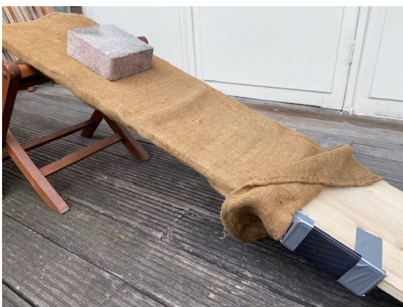
Figure 7.5: Jute was attached to the inclined wood plank. The tilt, measured by the phone, was increased until motion of the brick.
