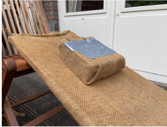
Figure 7.6: By wrapping a concrete brick with jute, a jute-jute interface is created.
