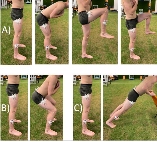
Fig. 3: Sensor-body calibration movements. Calibration A consists of a neutral pose followed by a bow, right thigh rise and left thigh rise. Calibration B consists of a neutral pose and a squat movement. Calibration C consists of a neutral pose and an inclined plank movement.
