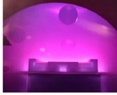
Figure 2.5: Secondary plasma around substrate holder for plasma obtained with an Ar-H 2 -SiH 4 gas mixture and an external rf bias additional to ETP-CVD.
