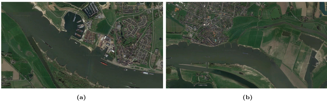
Figure 2.10: (a) An inland port ('vluchthaven') along the Dutch Upper Rhine near Lobith and (b) a sudden confinement of the floodplain width along the German Niederrhein at Rees. [source: Google Earth]
