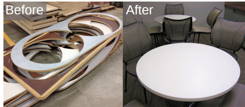
Figure 28- Reuse of existing core to create new tops. Source: (Remanufactured Office Furniture | Davies Office, n.d.).
