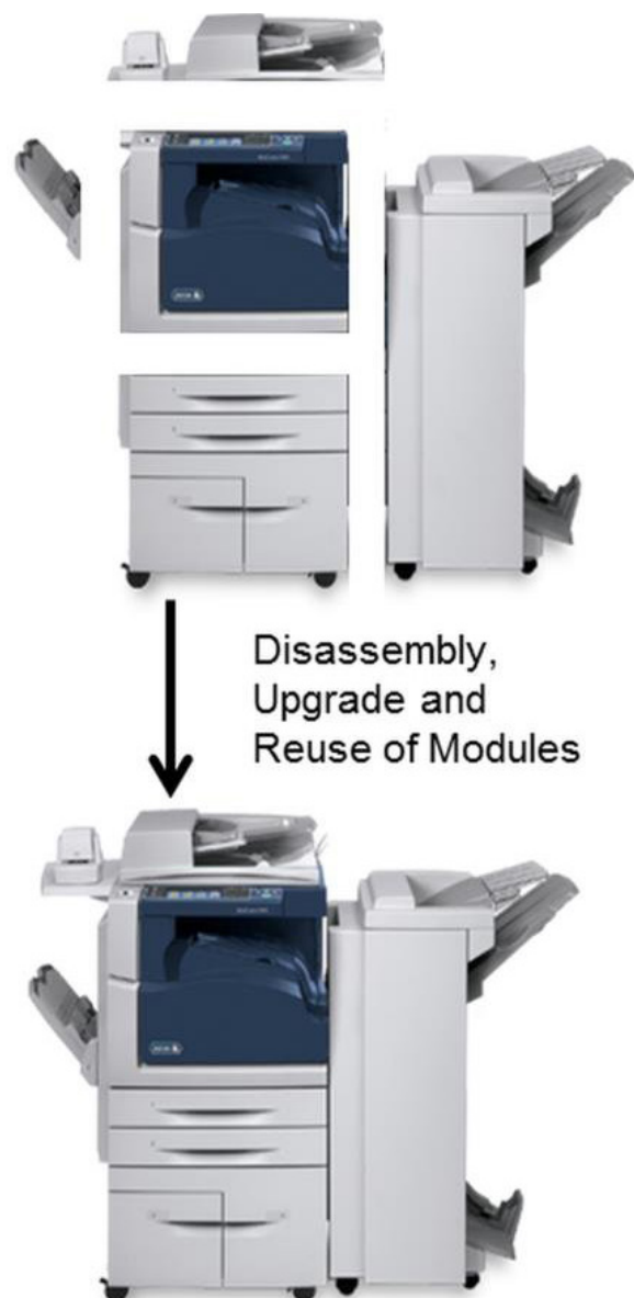
Figure37: Xerox reuses of existing core to create new tops. Source: (Telenko et al., 2016)
