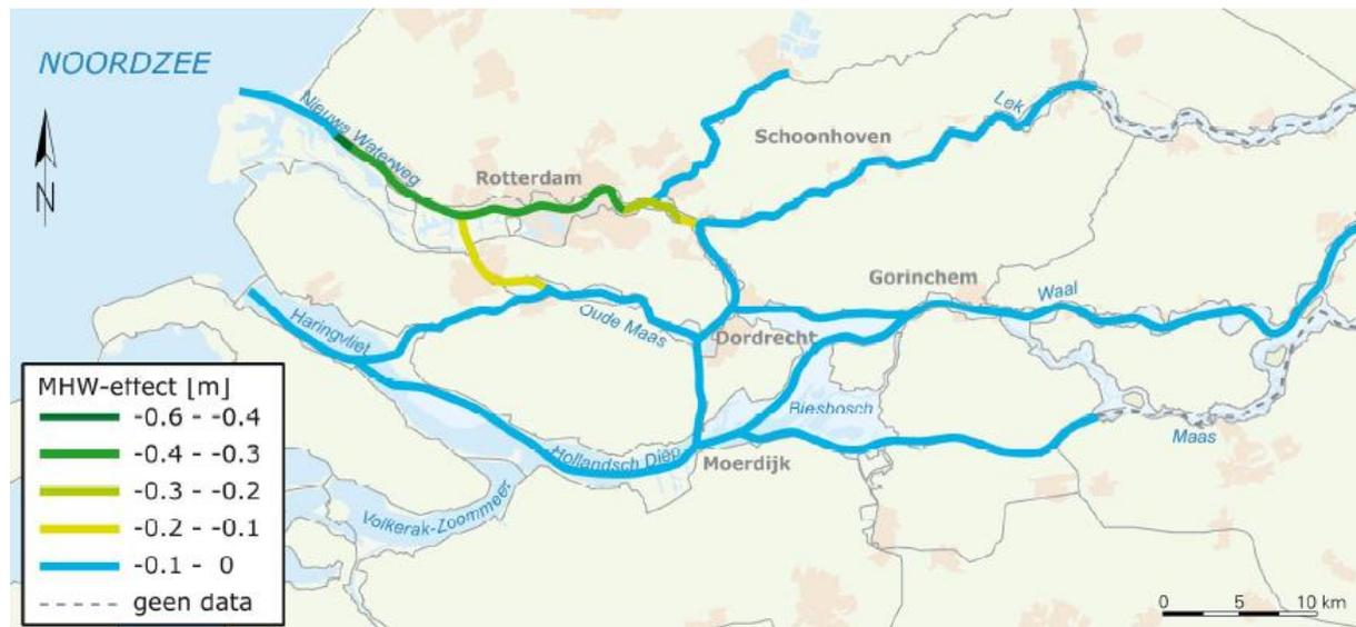
Figure 2.4 Spatial effect of a reduction in Maeslantkering failure probability on normative high water levels (Botterhuis et al., 2012)
