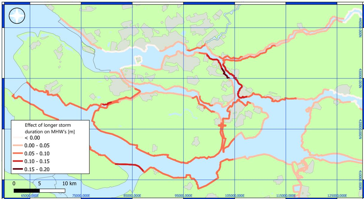
Figure 5.20 The effect of increased storm surge duration (27%) on MHW's in the current system (no Delta21)
