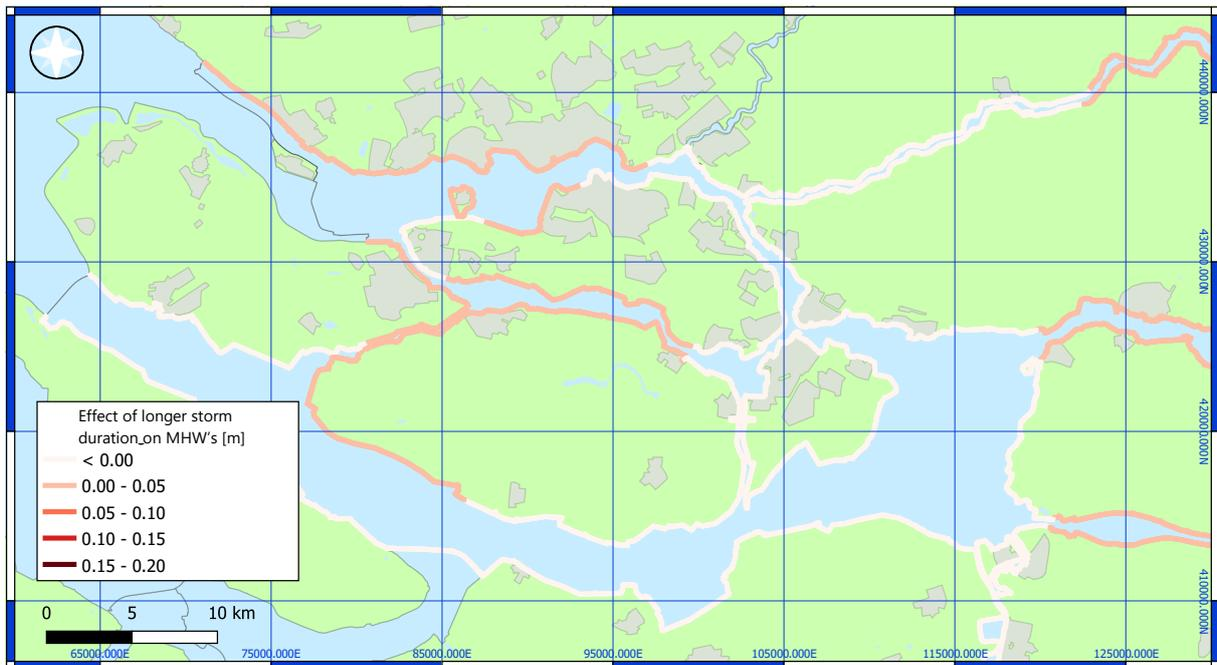
Figure 5.21 The effect of increased storm surge duration (27%) on MHW's in a system with the preliminary Delta21 configuration
