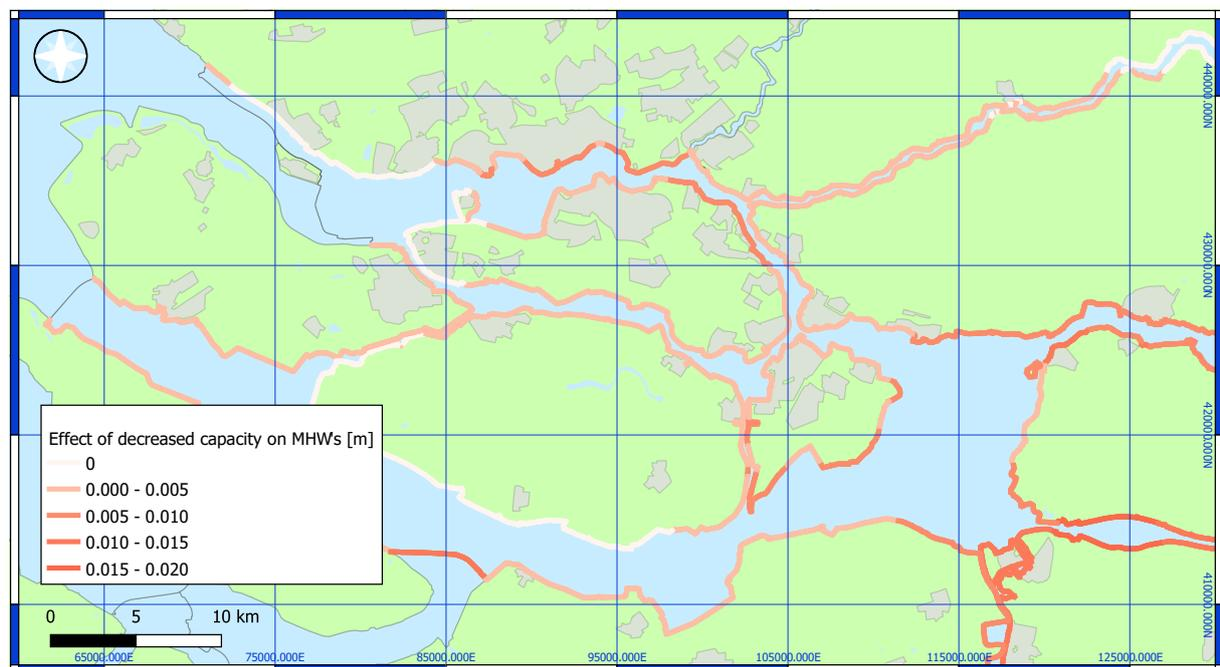
Figure 5.4 Effect of a reduced storage lake volume (25%) and reduced pump capacity (25%) on MHW's in the current climate
