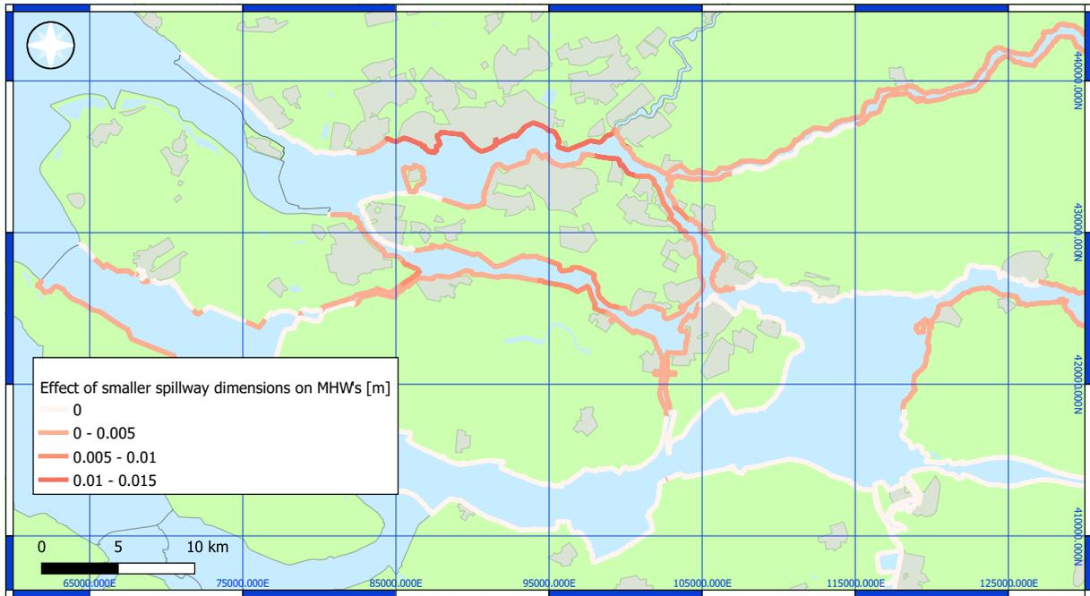
Figure 5.7 Effect of a reduced spillway width (25%) and raised sill height (1 m) on MHW's in the current climate
