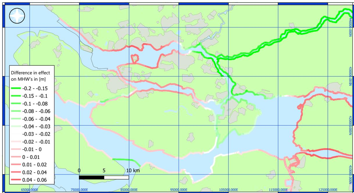
Figure 5.10 Difference in the effect of a changed discharge division at the Pannerdensch Kop on MHW's between the current and Delta21 systems
