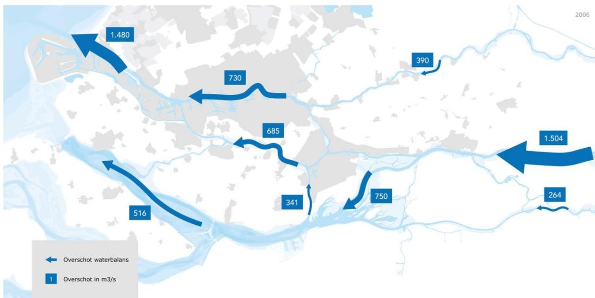
Figure B.12 Overview of average Rhine-Meuse delta discharges as of 2006 (Balla, et al., 2019)
