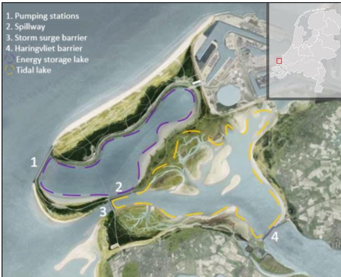
Figure 1.1 Overview of the most recent Delta21 components and layout. Adapted from Eeden (2021) and Verschoor (2023)
