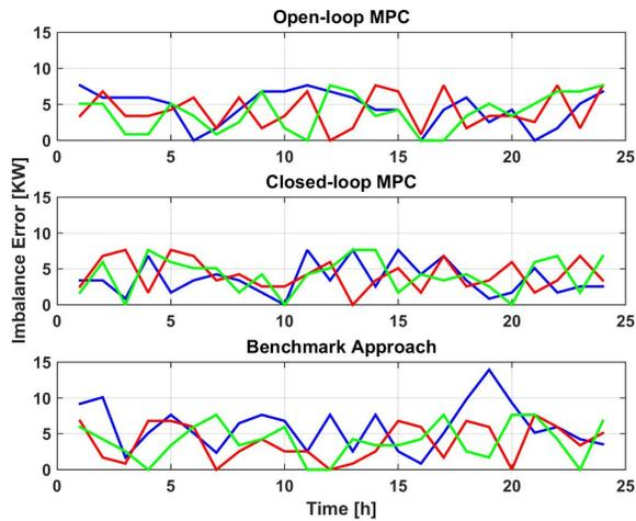
Fig. 2. Imbalance error trajectories. ‘Blue’ lines show to the imbalance error  $x_1$  in the first agent and  $x_2$  the imbalance error in the second agent is shown by ‘Red’ lines. ‘Green’ lines represent the imbalance error  $x_3$  in the third agent. The first, second and third sub-figures are related to the results of open-loop MPC, closed-loop MPC considering affine uncertainty feedback, and the Benchmark approach, respectively.
