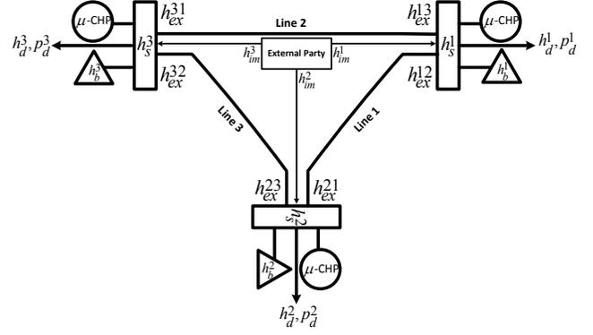
Fig. 1. Three-agent (households, greenhouses) thermal grid example. Each agent has a  $\mu$ -CHP, a boiler and a thermal storage.  $h_s^1, h_s^2, h_s^3$  are related to the local thermal storage in agent one, two and three, respectively. There are also three lines between agents indicating that thermal energy exchange is possible. It is considered to have an external party available for all agents to provide thermal energy.
