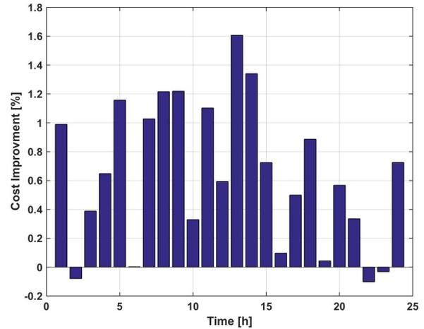
Fig. 4. Normalized relative cost improvement of the closed-loop MPC approach (affine uncertainty feedback) over the Benchmark approach.
