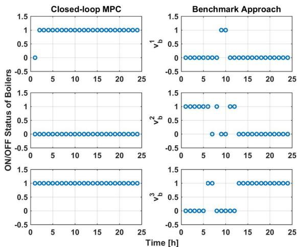
Fig. 3. ON/OFF status of boilers. The first, second and third sub-figures are related to agent 1, 2, and 3, respectively. The sub-figures on the left are the results of closed-loop MPC considering affine uncertainty feedback, and the sub-figures on the right are the results of the Benchmark approach.
