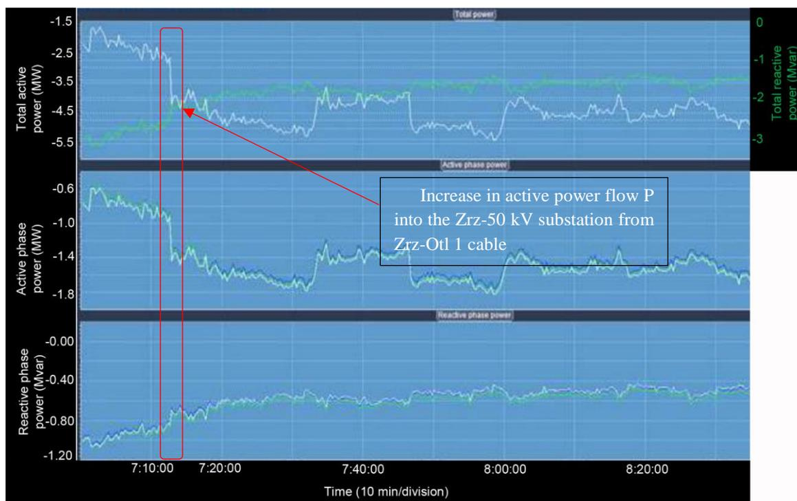
Figure 5-5: Zrz-Otl 1 PMU log showing the power flows on the Zrz-Otl 1 cable
