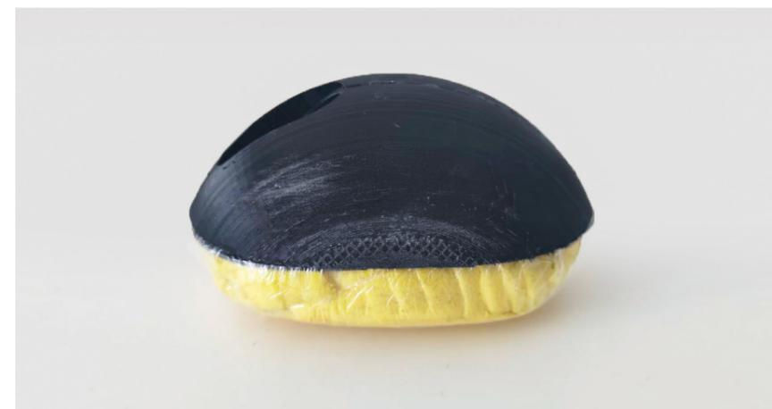
Figure 64 - We printed a shell using a FDM printer. On the bottom we attached a piece of foam shown in figure 63.
