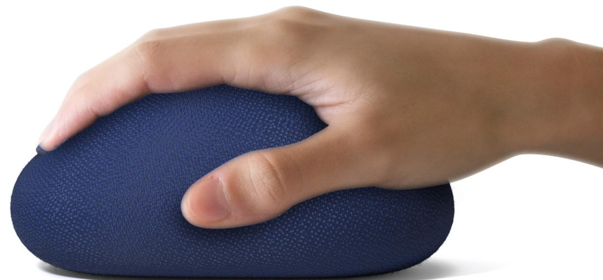
The Somnox Mini teaches its users how to perform the exercise by providing a physical breathing guide. The device has a plate that moves up and down, simulating a natural inhalation and exhalation. By resting the hand on the top surface, the user can feel a rising and falling sensation and breathe along with it.
