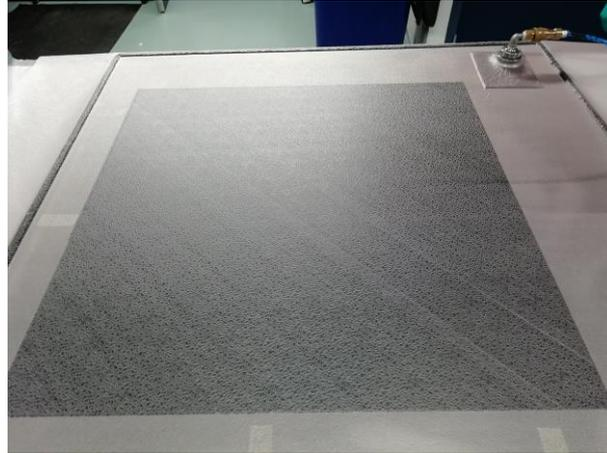
Fig. 3.2: Making composite plate by hand lay-up method.
