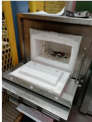
Fig. 3.7: Heating specimens in muffle furnace.
