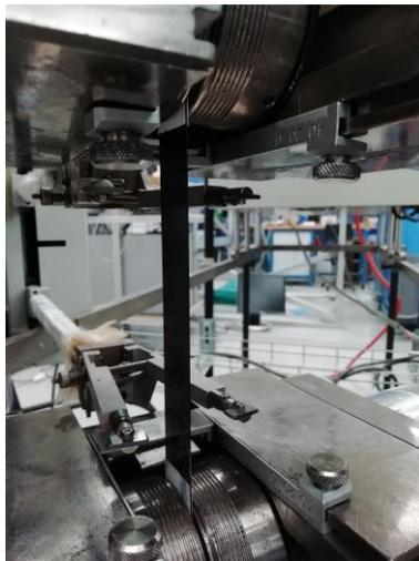
Fig. 3.22: Using extensometer to measure strain in the stiffness tests.
