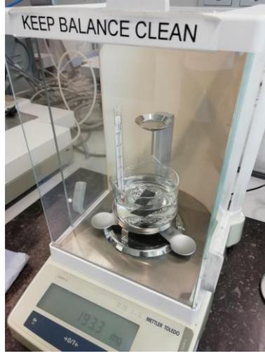
Fig. 3.6: Weighing specimens in air and in water.
