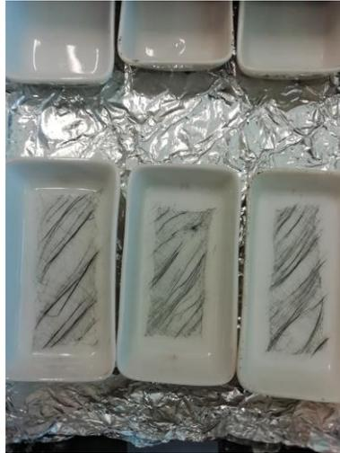
Fig. 3.9: The fibres were left behind in crucibles after heating.
