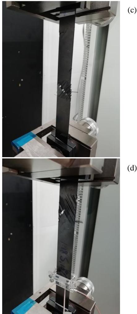
Fig. 3.18: Ultimate tensile failure tests of specimens No. 15 to 18 (from (a) to (d)).
