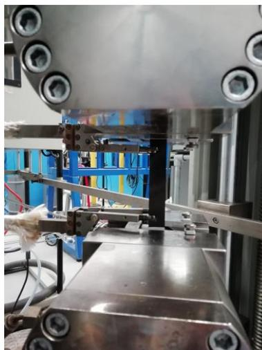
Fig. 3.26: Stiffness tests of wet specimens (e.g., specimen No. 18).
