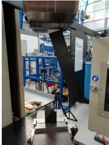
Fig. 3.25: Failure tests of wet specimens (e.g., specimen No. 1).
