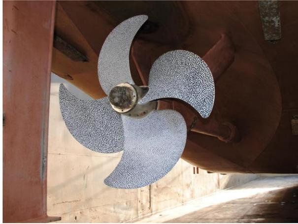
Fig. 1.1: Composite propeller used in test (Photo: MARIN).
