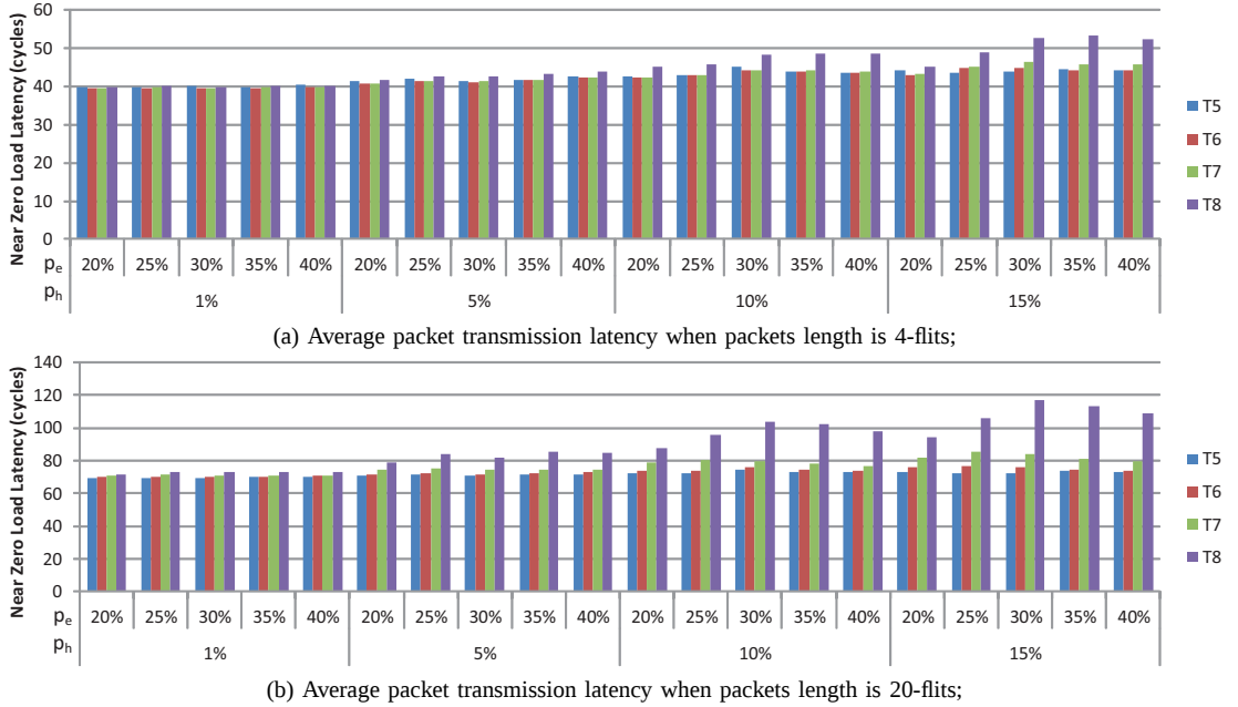
Fig. 12. The system average packet transmission latency when deactivate links with high fault level with different threshold.
