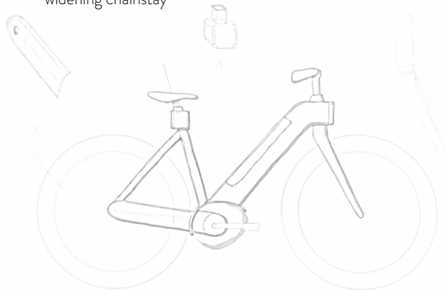
3 Rectangle lower tube profile, with straight seat tube and a wide, straight chainstay
