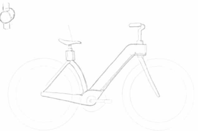
2 Round lower tube profile, with curved seat tube and more narrow, but widening chainstay
