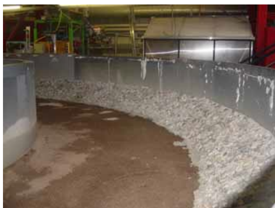
Figure 5: Flume in Lausanne, with an inclined rough outer-bank, as used for the experiments of Duarte [2008].
