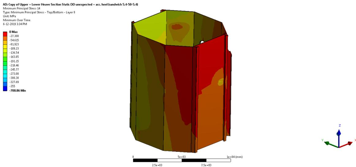
Figure 6.8 Minimum principle stress (upper part)
