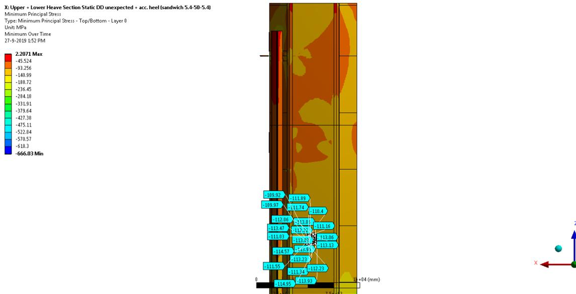
Figure 6.3 Minimum principle stress
