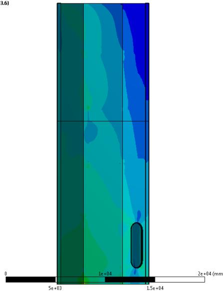
Figure 6.14 Von Mises stress (back view)
