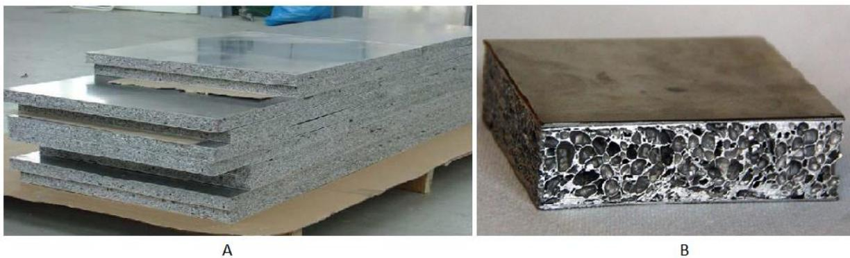
Figure 2.1 Steel Aluminium Foam Sandwich Panel [5][6]
