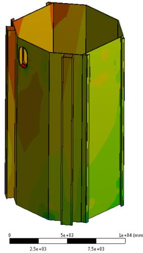
Figure 6.9 Minimum principle stress (lower part)
