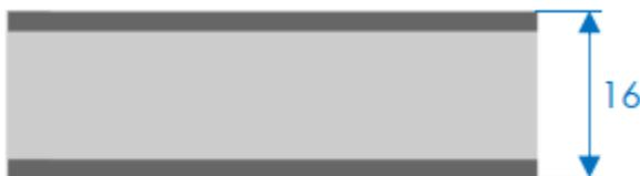
Figure 3.17 Sandwich cross-section
