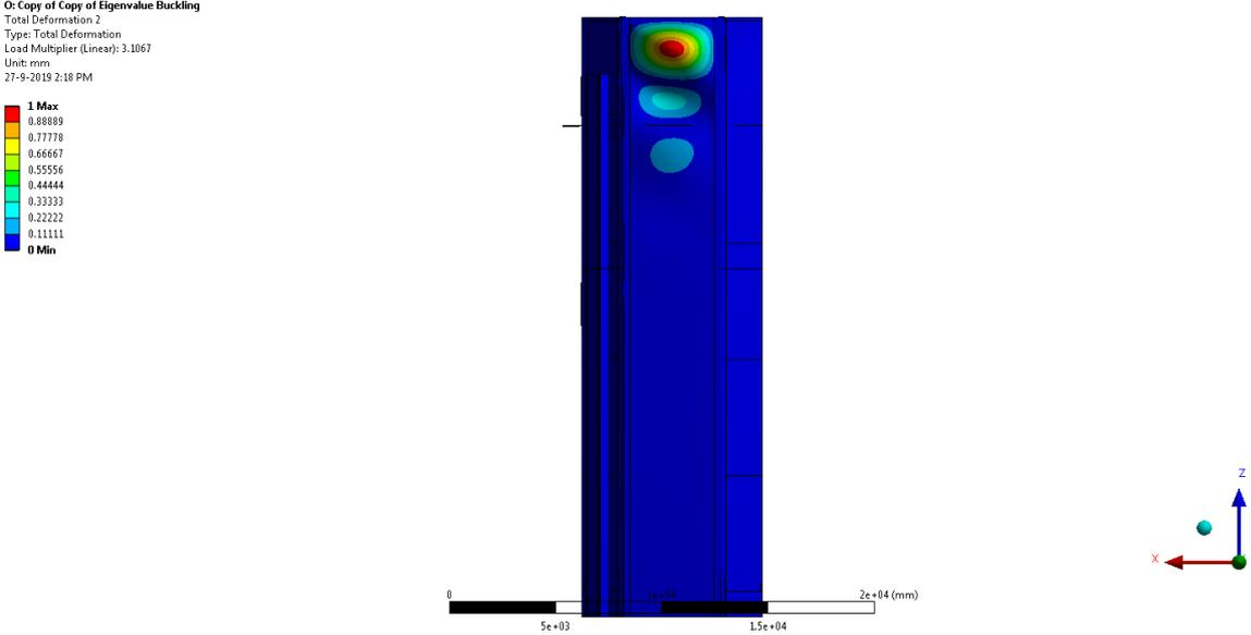
Figure 6.11 Buckling of heave section
