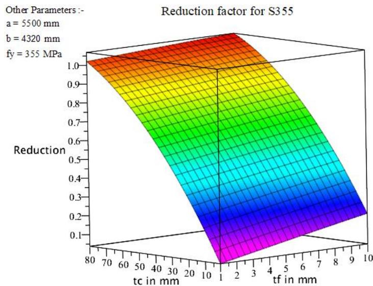
Figure 5.6 Reduction factor for a sandwich with faceplates S355
