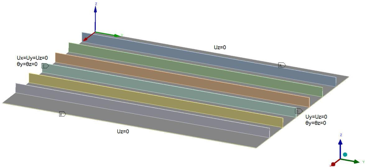
Figure B.4 Boundary conditions of sandwich panel
