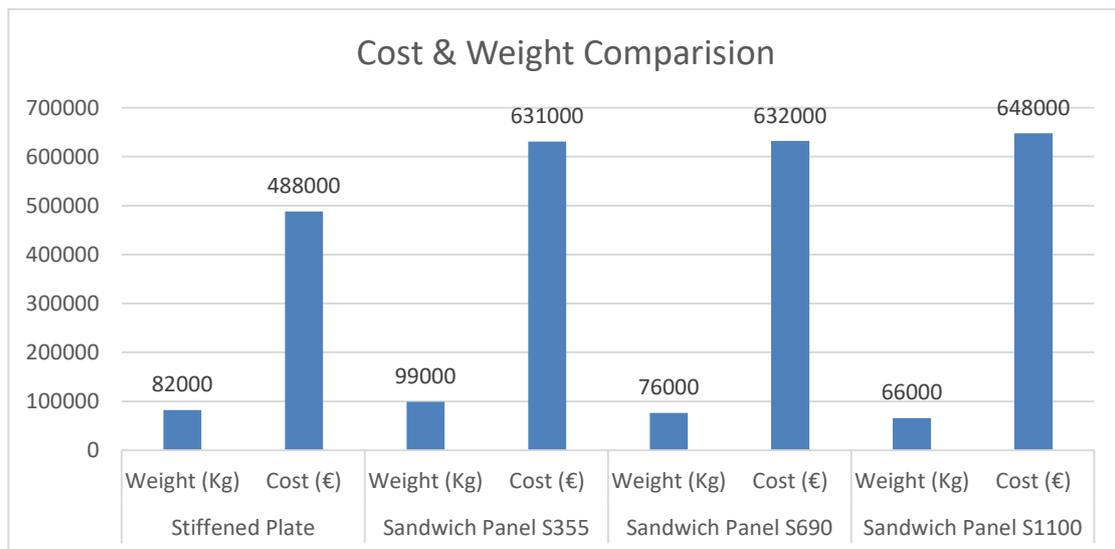
Figure 6.31 Cost & weight Comparison
