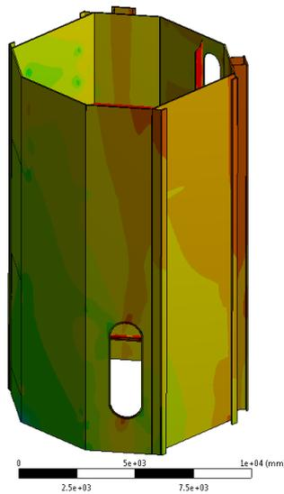
Figure 6.28 Minimum principle stress (lower part)
