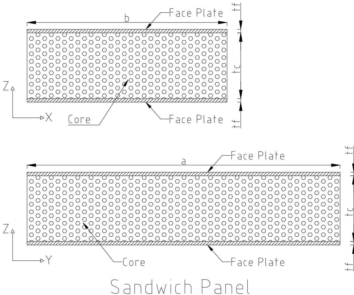
Figure 4.3 General configuration of the sandwich panel
