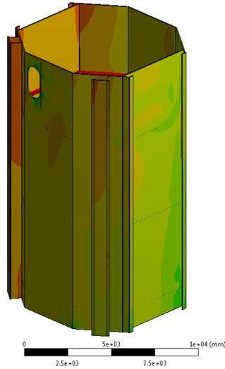
Figure 6.27 Minimum principle stress (lower part)
