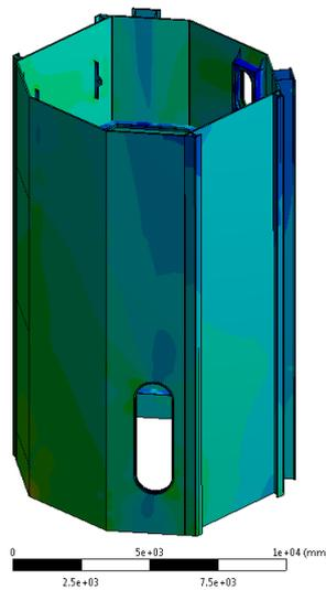
Figure 6.19 Minimum principle stress (lower part)
