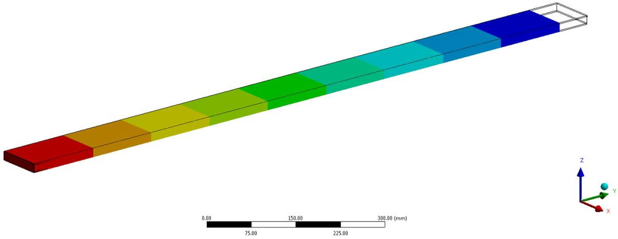
Figure 3.8 In-plane displacement of sandwich panel
