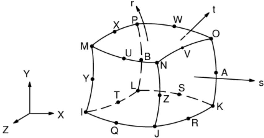
Figure D.10 ANSYS element type SOLID186 [9]
