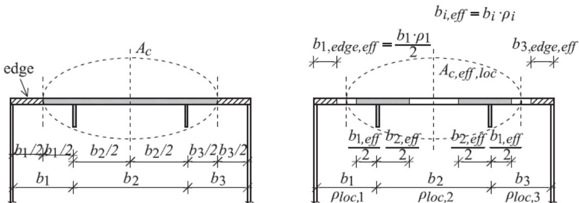
Figure 4.2 Stiffened plate under uniform compression [11]
