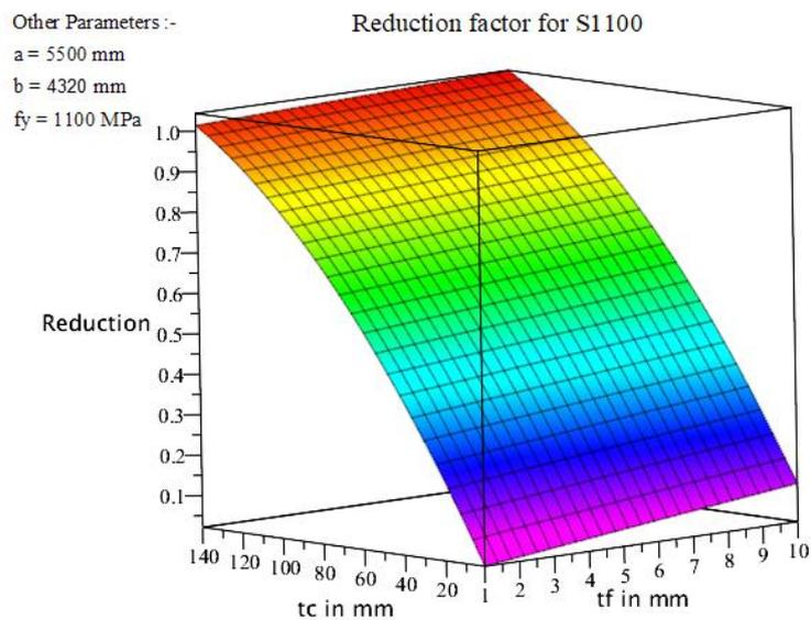
Figure 5.8 Reduction factor for a sandwich with faceplates S1100
