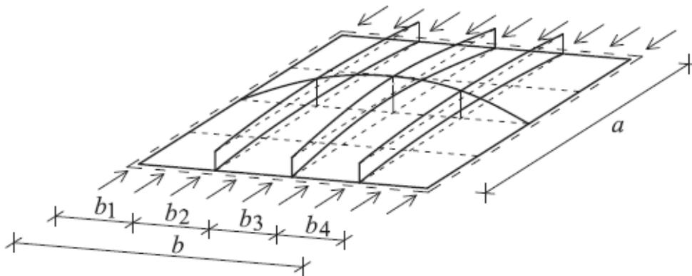
Figure 4.1 Plate like buckling of a stiffened plate [11]
