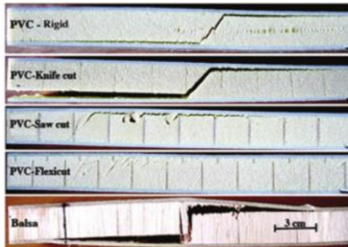
Core failure in four point bending test for different core types.
