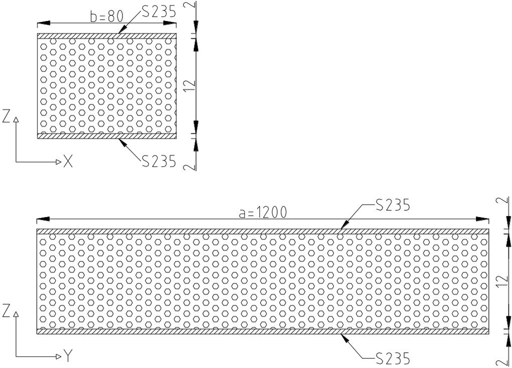
Figure 2.25 Sandwich panel used in the report by Havel [14]
