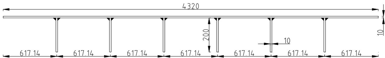
Figure C.1 Cross-section of stiffened plate
