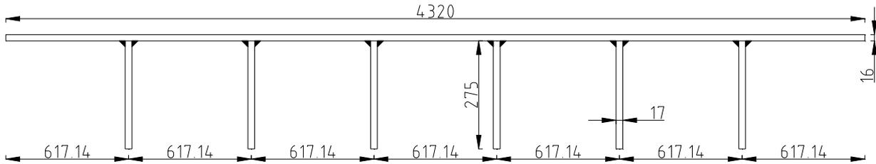
Figure G.2 Cross-section of stiffened plate
