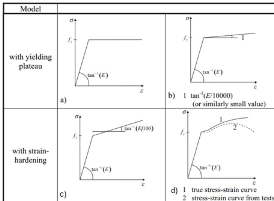
Figure 3.1 Modelling of material behaviour (from EN 1993-1-5) [49][11]
