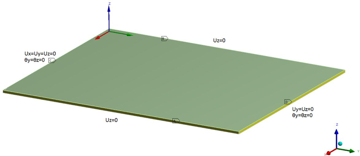
Figure D.12 Boundary conditions of sandwich panel
