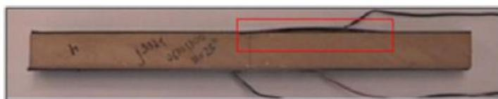
(a) Delamination failure mode after impact.
