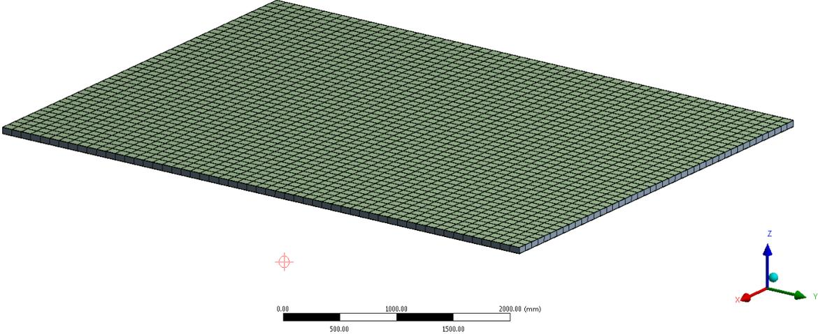
Figure D.11 Sandwich Meshing.
