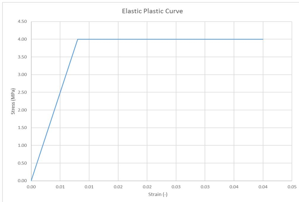
Figure 3.4 Aluminium material model Bi-linear
