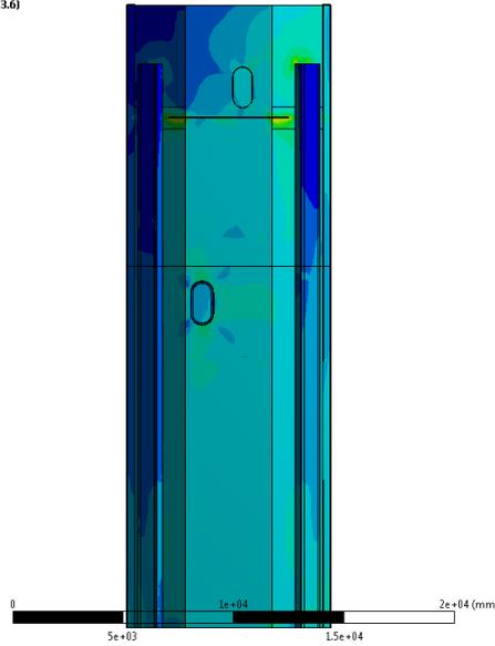
Figure 6.13 Von Mises stress (front view)
