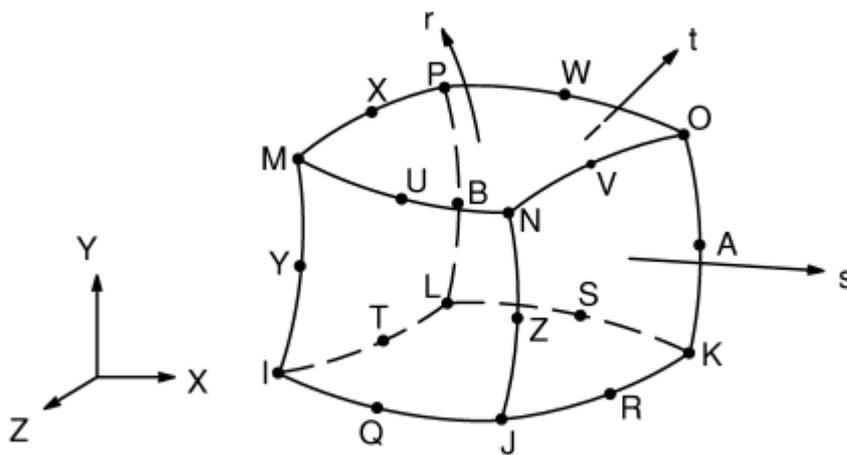
Figure A.2 ANSYS element type SOLID186 [9]
