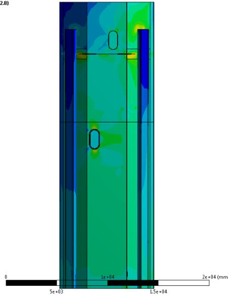
Figure 6.22 Von Mises stress (front view)
