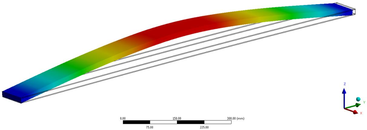
Figure 3.9 Out-of-plane displacement of sandwich panel
