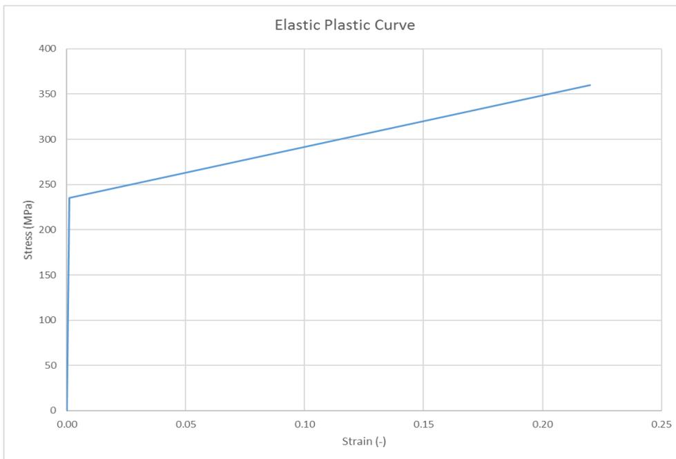
Figure 3.3 Steel material model Bi-linear
