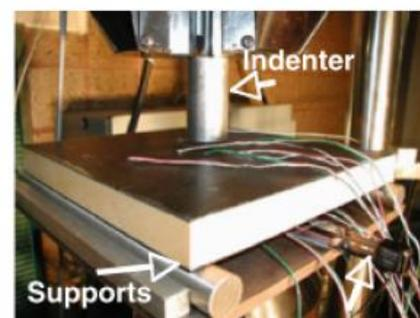
(b) Impact test setup.
