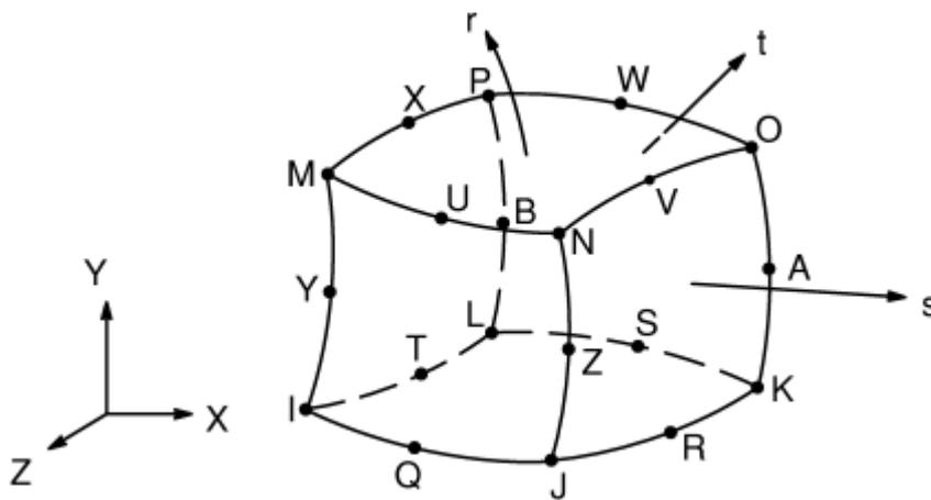
Figure D.2 ANSYS element type SOLID186 [9]
