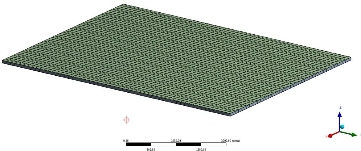
Figure D.3 Sandwich Meshing.
