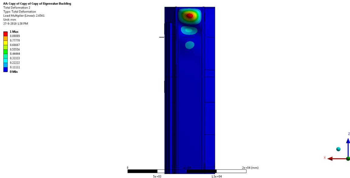
Figure 6.20 Buckling of heave section
