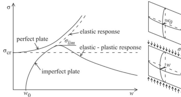
Figure 2.21 Post-critical response of slender plates subjected to compression [11]
