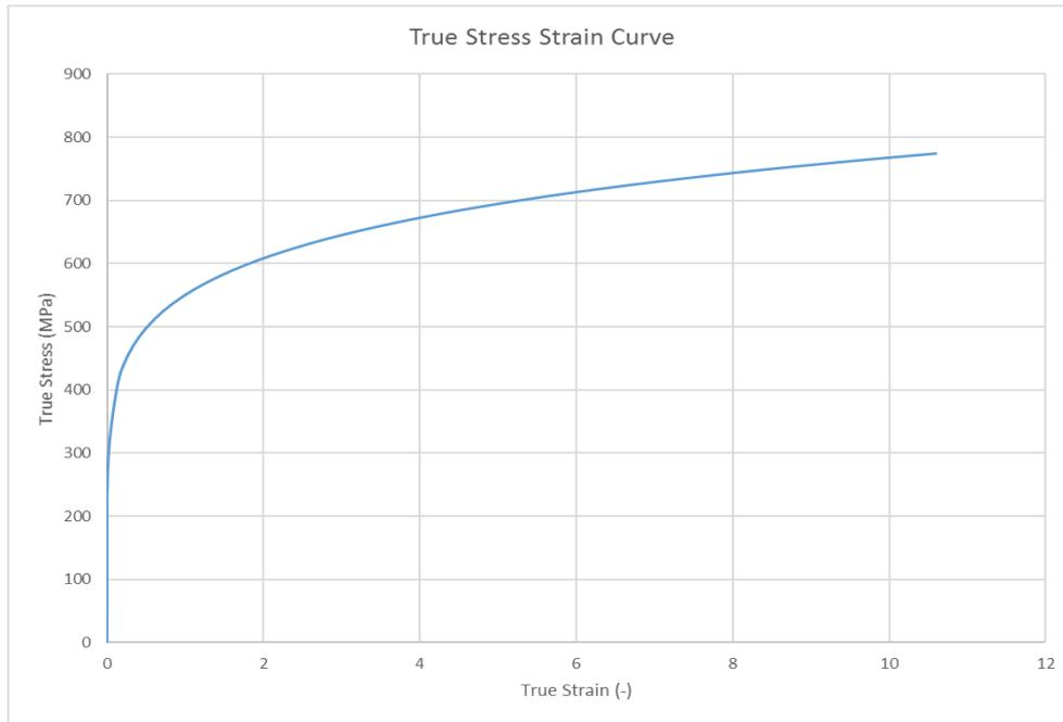
Figure 3.2 Steel material model Multi-linear
