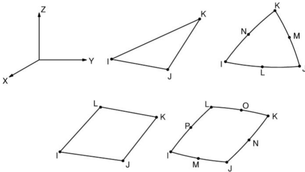
Figure 2.16 Shell Elements Triangle and Rectangle [9]
