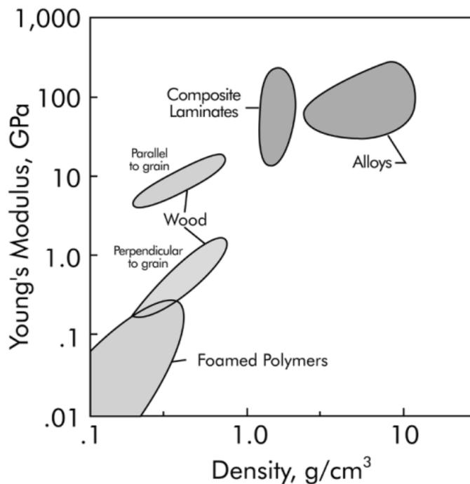
Figure 2.3 Modulus density chart for various classes of materials. After Ashby 1999 [8]
