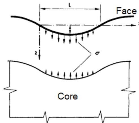
Figure 3.23 Stress between the faceplate and supporting elastic medium (core)
