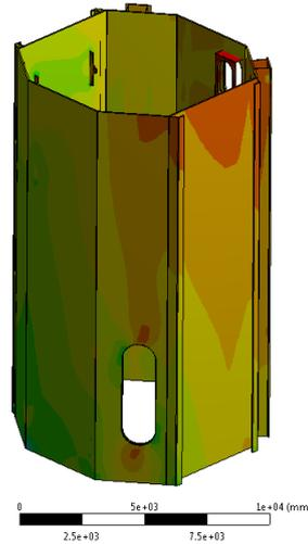
Figure 6.10 Minimum principle stress (lower part)
