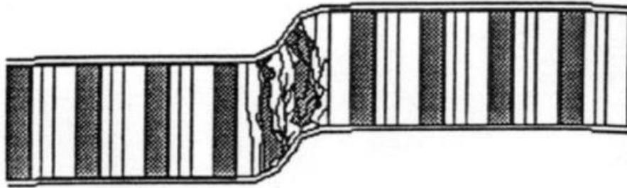
Figure 4.5 Core shear instability [3]
