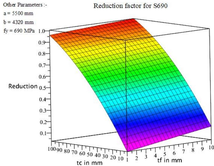
Figure 5.7 Reduction factor for a sandwich with faceplates S690
