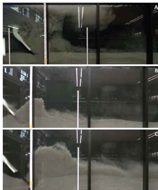
Figure 3: Set of preliminary experiments: (a) Experiment 1 - peak of discharge; (b) Experiment 2 - low discharge; (c) Experiment 3 - intermediate discharge.
