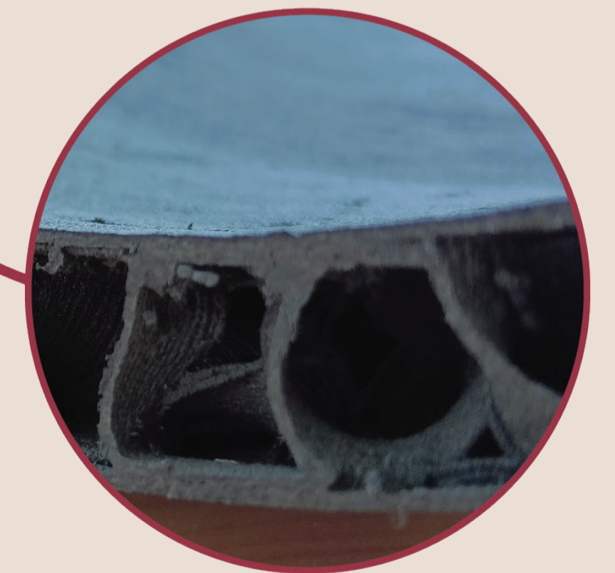
Foaming TPU printed at 240°C with 12% gyroid infill.
