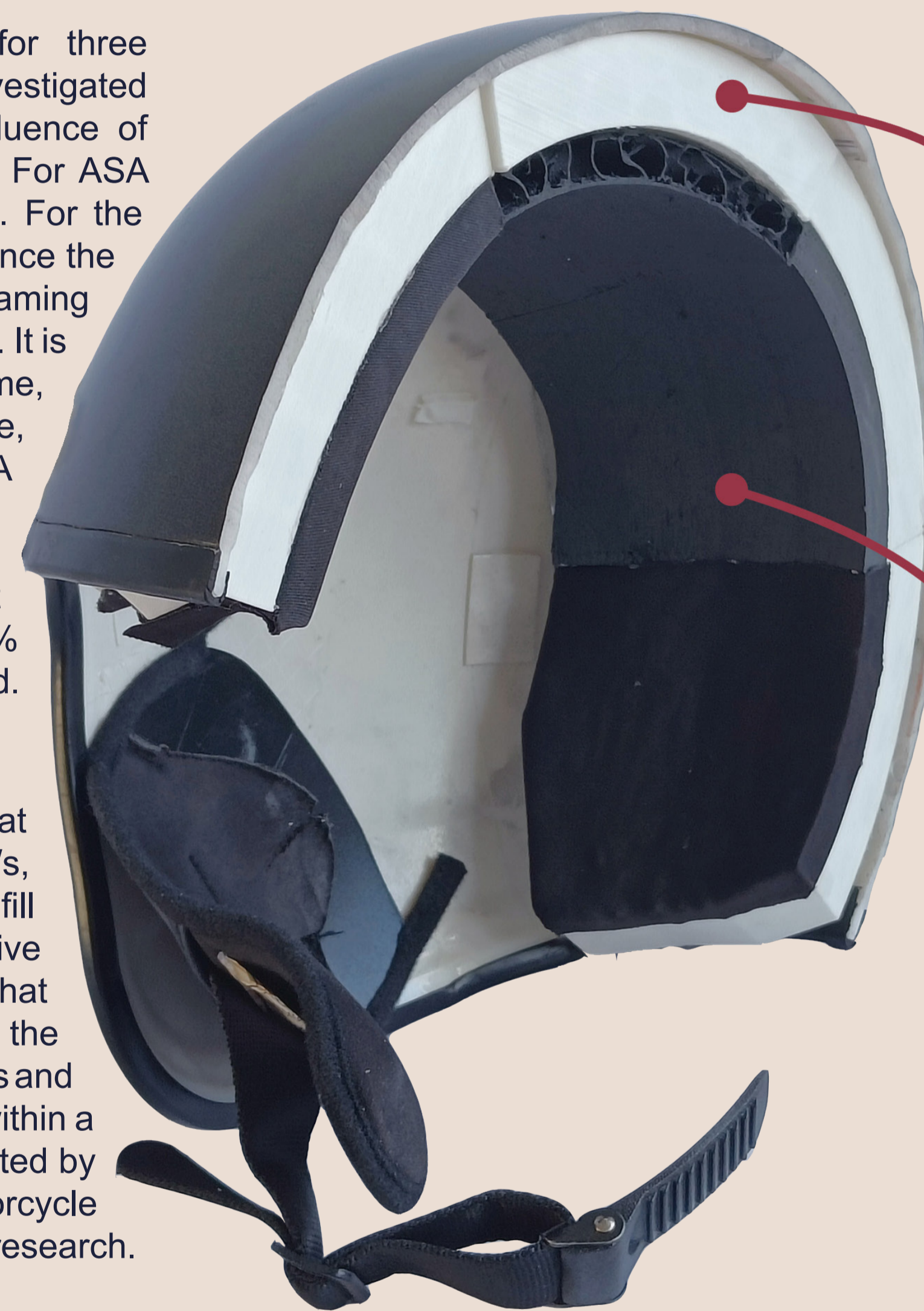
Motorcycle helmet with 3D printed foaming materials as impact and comfort liner
