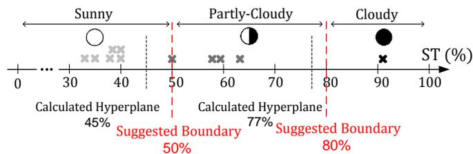
Fig. 4. Proposed shading classification boundaries for PV modules
