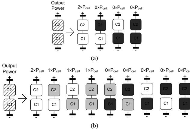
**Fig. A.1.** Graphical demonstration of  $ST$  formulation procedure: (a) PV module with two series-connected cells and two possible irradiation levels (0 and 1 kW/m<sup>2</sup>) which results in total 2<sup>2</sup> working conditions, (b) PV module with two series-connected cells and three possible irradiation levels (0, 0.5, and 1 kW/m<sup>2</sup>) which results in total 3<sup>2</sup> working conditions. Output power of PV modules at each working condition is also depicted.
