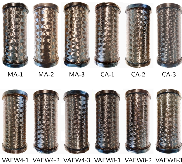
Fig. 2. Filament-wound cylinders used in the imperfection measurements.
