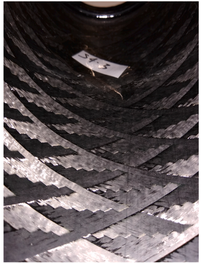
Fig. 16. Inner surface of filament-wound cylinder VAFW4-3. The smooth mandrel produces a significantly smoother inner surface on the cylinder compared to the outer surface.
