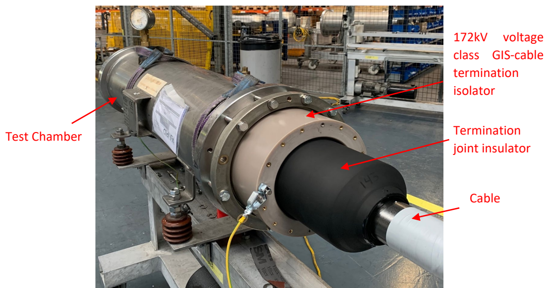
Figure 6.23: 172kV GIS-Cable termination test setup
