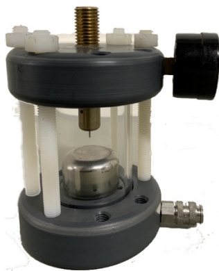
Figure 5.2: Test cell with protrusion fixed on a conductor depicting Corona
