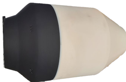
Figure 6.18: Stress Cone utilised for the test
