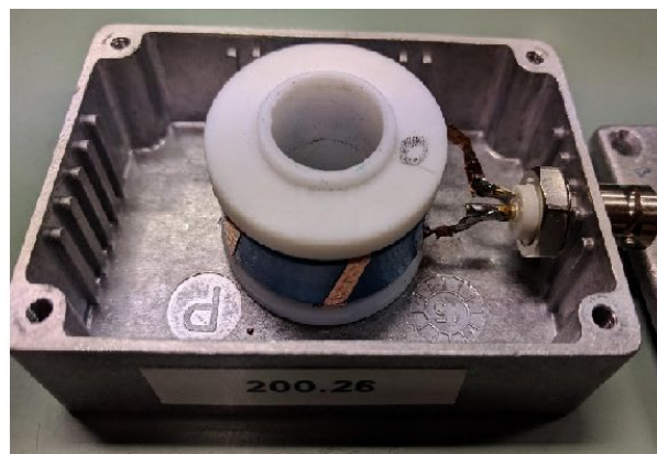
Figure 5.9: HFCT sensor with a gain of 9.1mV/mA
