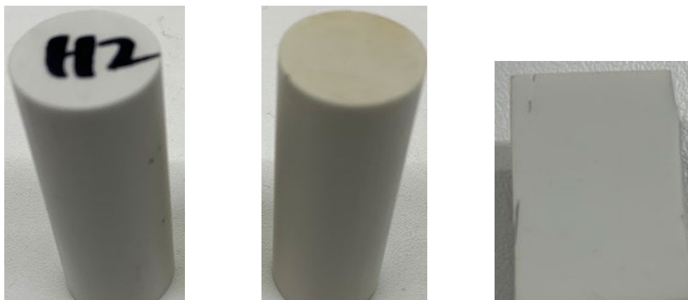
Figure 4.8: Epoxy with Al 2 O 3 filler (a) aged in oven with ambient air (b) aged in gas (c) cutsection of epoxy aged in gas
