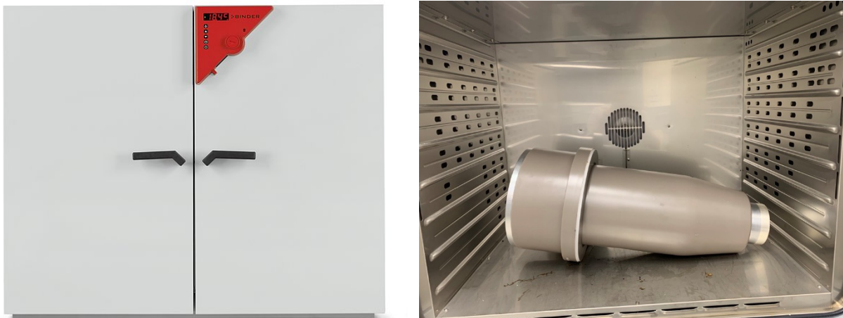
Figure 4.6: BINDER BD 400 and the chamber with epoxy inside the oven
