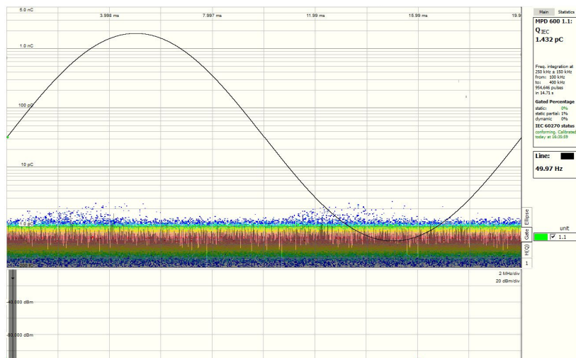
Figure 6.24: PRPD at 261kV
