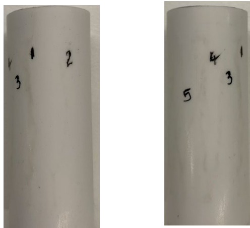
Figure 4.21: Flashover traces at 3 bar in C 4 F 7 N/CO 2
