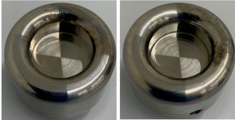
Figure 4.22: Crates on the electrode after LI tests
