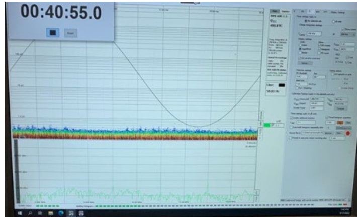
Figure 6.22: PRPD pattern of the test at 220kV
