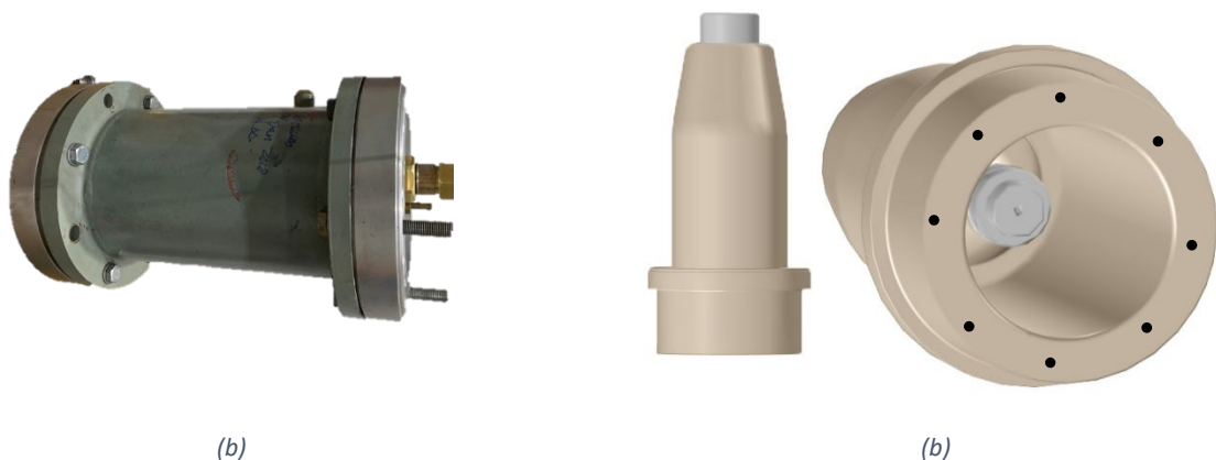
Figure 4.4: Ageing chambers (a) stainless steel chamber (b) GIS-cable termination
