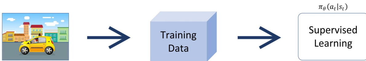
Figure 2.1: A simplified depiction of the Behavioural Cloning approach (adapted from Pérez-Dattari (2019)), where demonstrations are acquired from a domain expert as a dataset of labelled state-action pairs and a novice agent is trained in a supervised fashion to imitate the performance of the expert.
