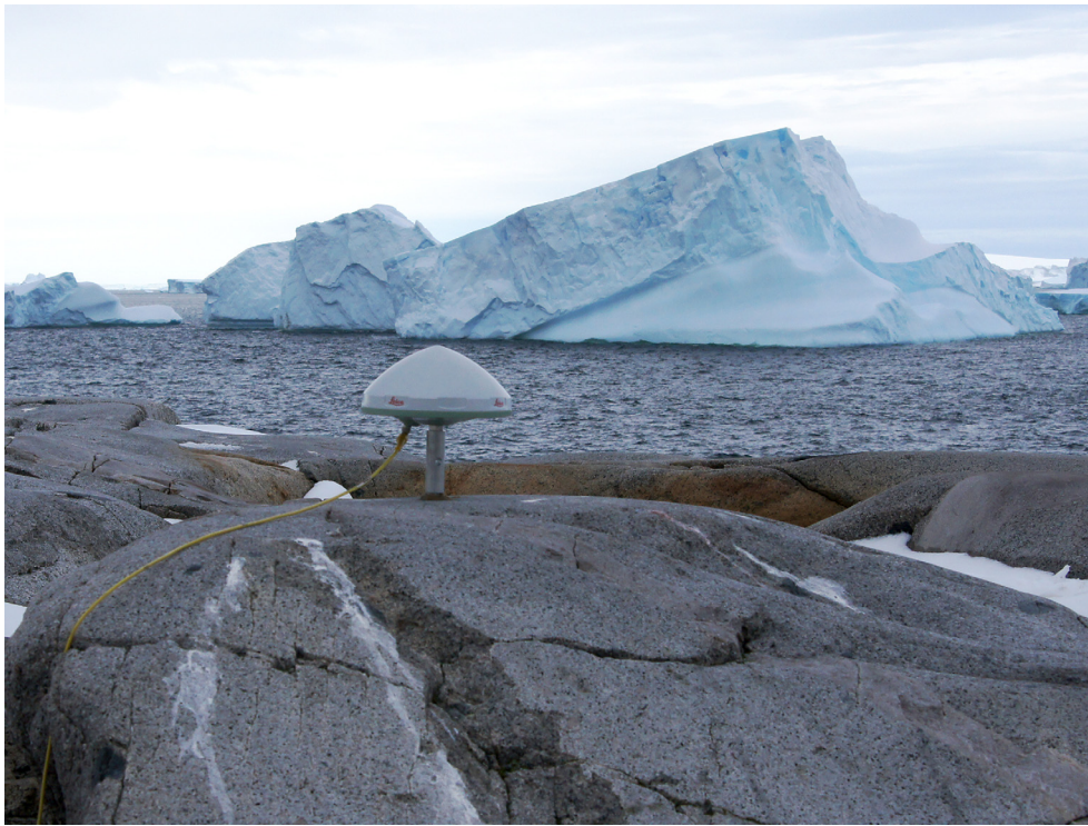
Fig. 2. Example of a GNSS campaign site: Backer Islands, Pine Island Bay, West Antarctica. Image credits: M. Scheinert.
