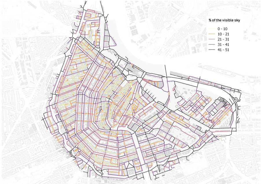
Figure 4.26: Percentage of the visible sky per street segment in the center of Amsterdam.
