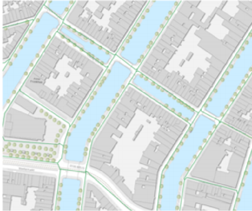
Figure 4.14: Extraction of the centreline from the polygon.
