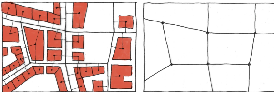
Figure 3.9: Correction of the simplified street network based on the building footprints.
