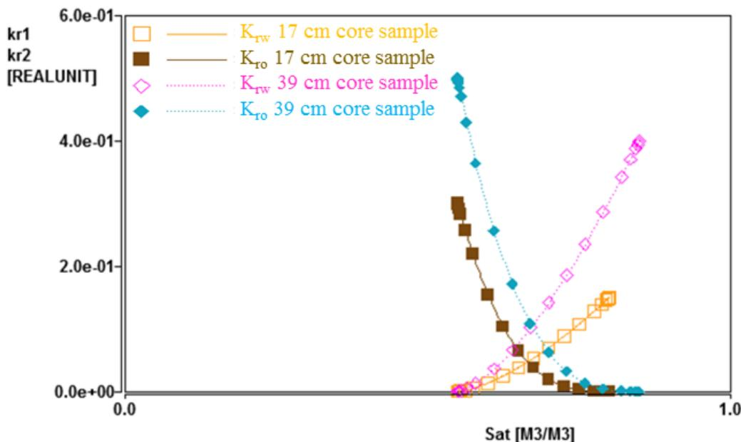
**Figure 4** Comparison of relative permeability at two different cores (17 cm vs 39 cm) during chemical flooding.
