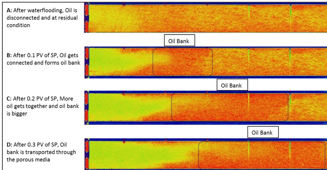
**Figure 3** Oil Bank build up process in the core (Core Length is 38 cm, core diameter is 3.8 cm, Red color indicates oil, green is the surfactant polymer).
