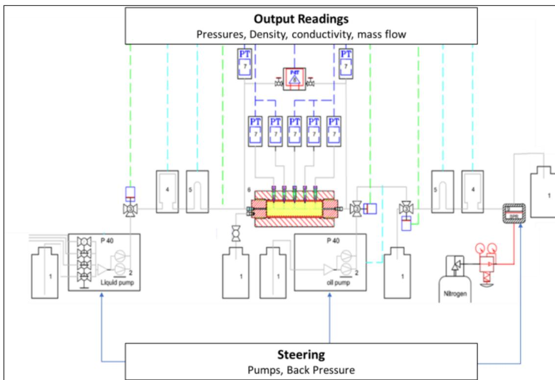
**Figure 1** Schematic design of the core flow setup. The numbers correspond with the set-up description here below.
