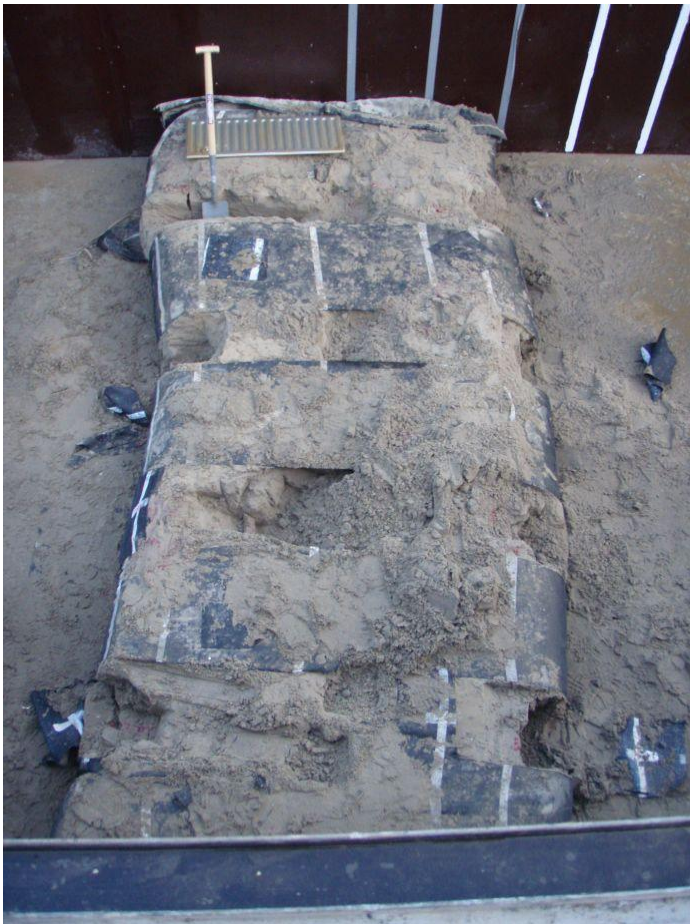
Photo 32: After examining the geotextile tube (F1)
