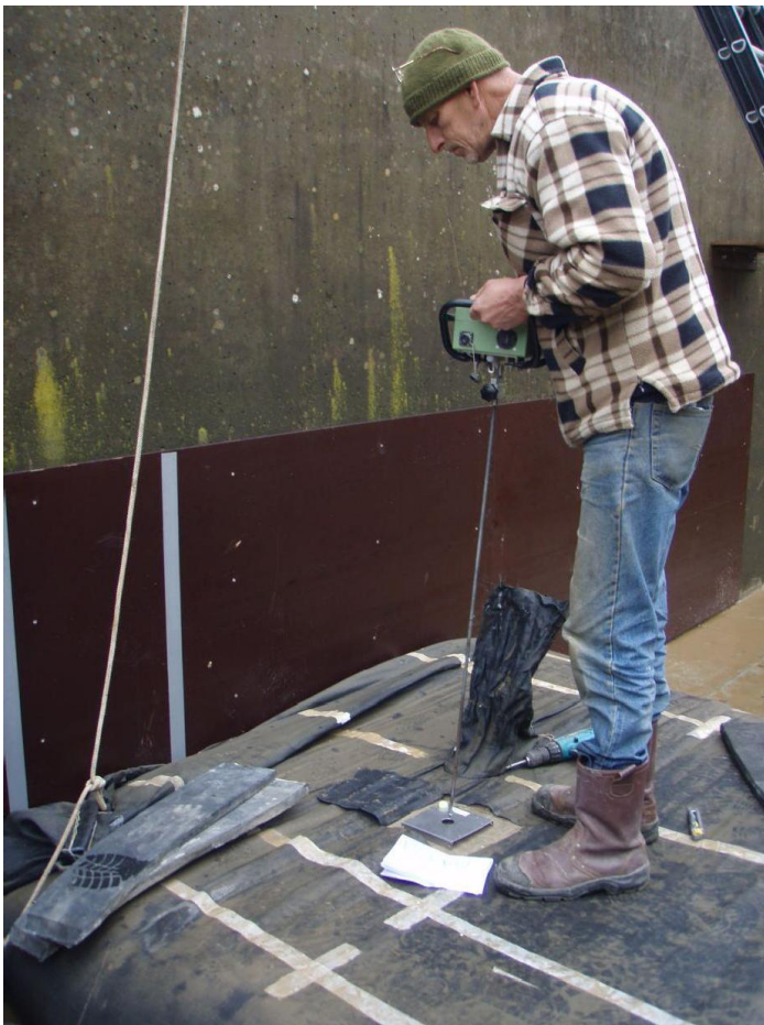
Photo 25: Measurements with Penetrologger
