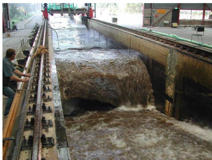
Wave impact at a placed block revetment
