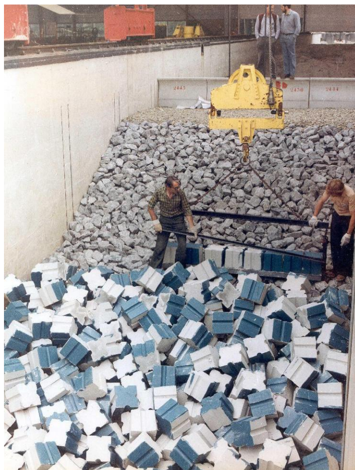
Placement of antifer cubes in a breakwater model in the Delta flume
