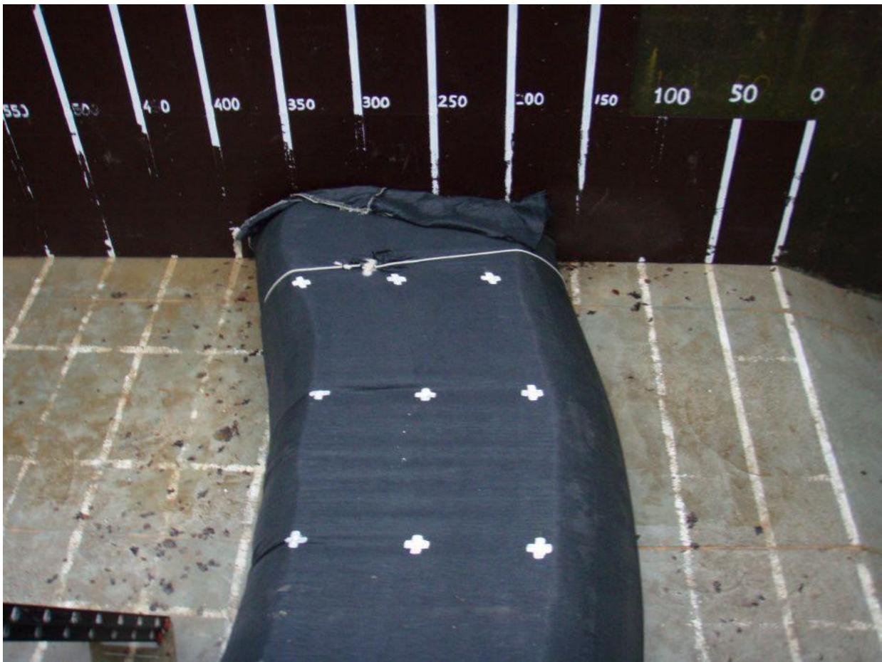
Photo 49: Deformed geotextile tube after test series F5-6
