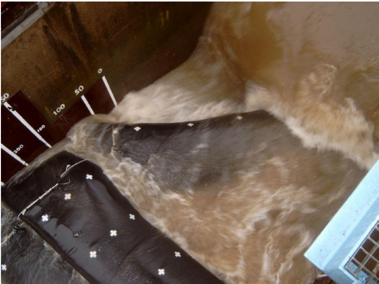
Photo 44: Sliding of geotextile tube during test series P3-9
