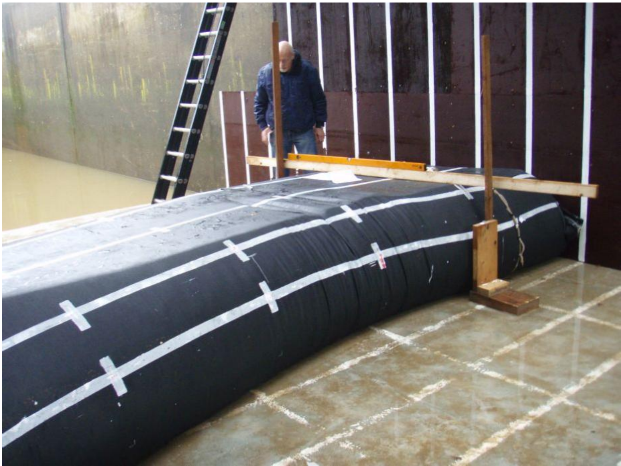
Photo 35: Measuring height geotextile tube after test series F3-9
