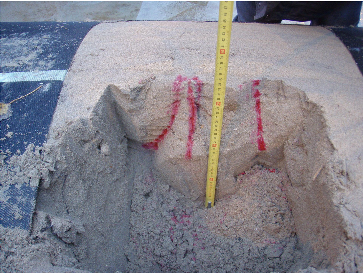
Photo 54: Color injection test series F4. Injection at line3, point 5
