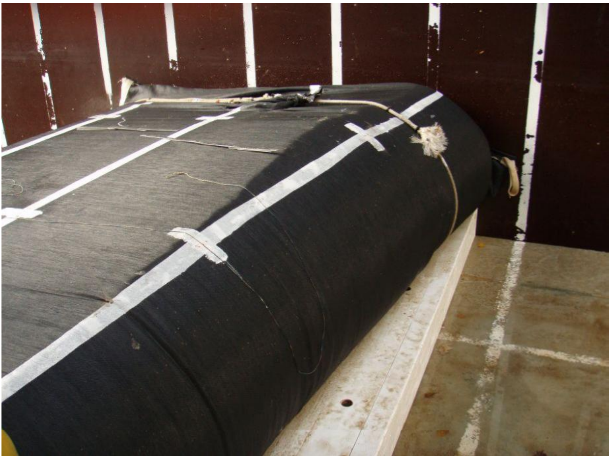
Photo 40: Geotextile tube partly on bar after test series T1-9
