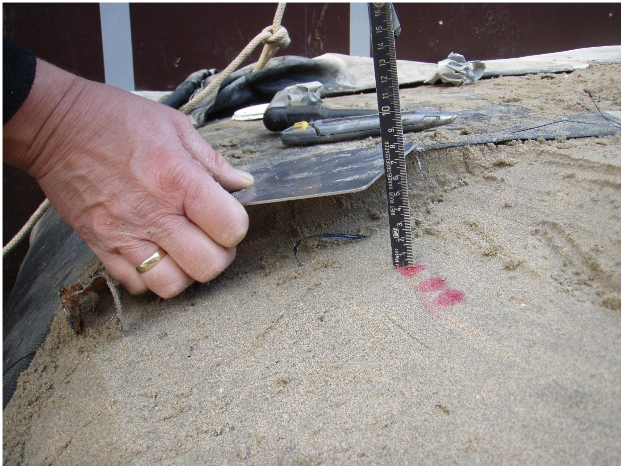
Photo 50: Color injection test series F1. Injection at line 4, point 3
