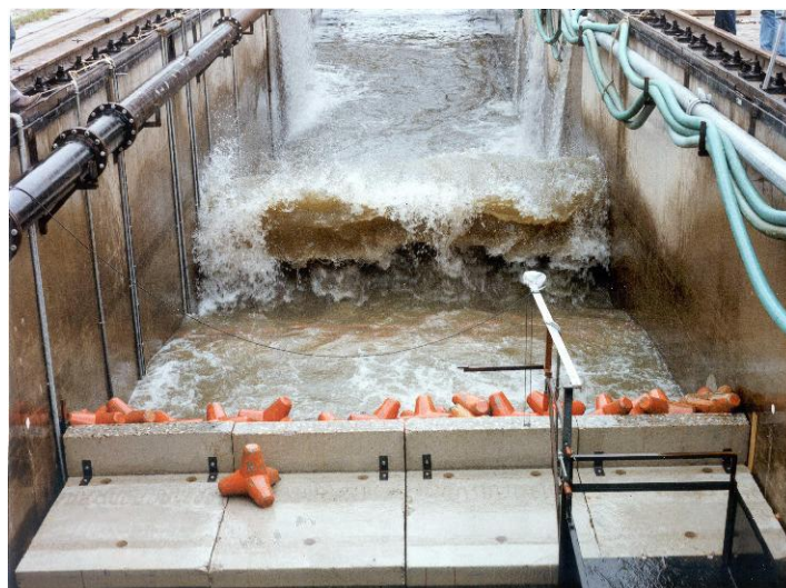
Typical breakwater model with tetrapods, measurements carried out: stability, overtopping discharge and overtopping events, waves
