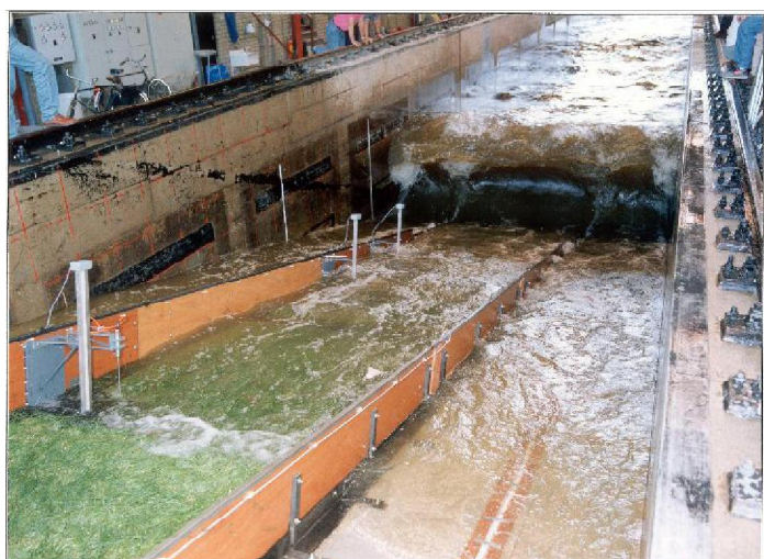
Measurement of erosion resistance of grass on a dike
