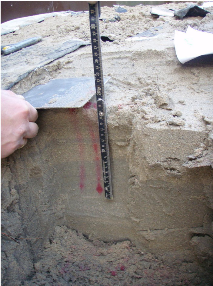
Photo 51: Color injection test series F1. Injection at line 4, point 3
