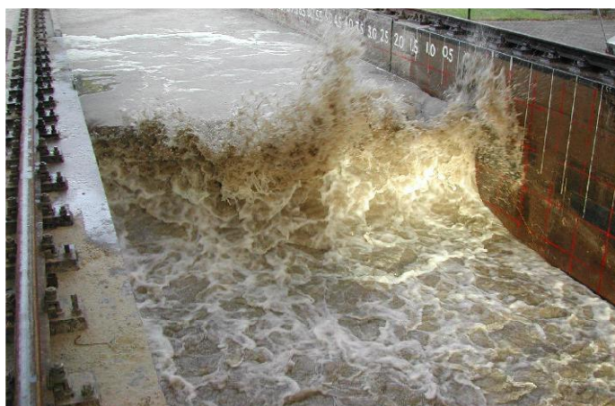
Wave impact during dune erosion test
