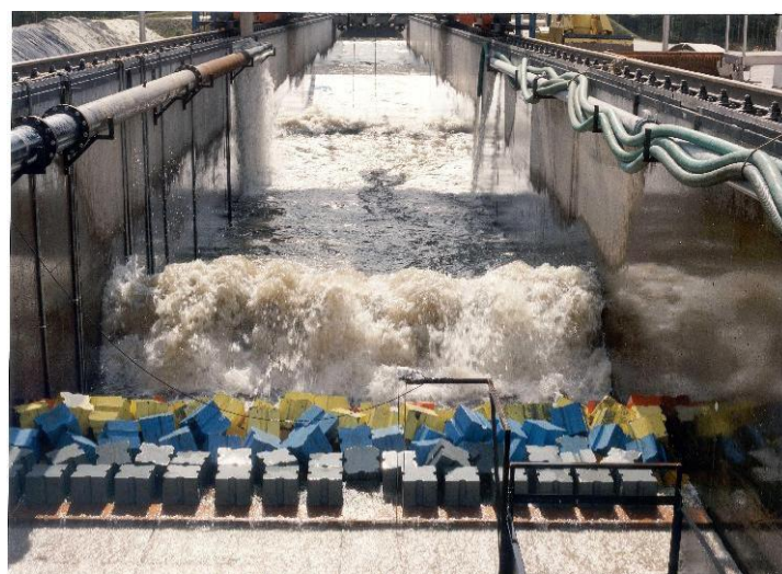
Model of a breakwater in the Delta flume
