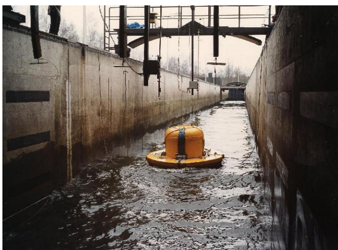
Testing and calibrating a wave gauge
