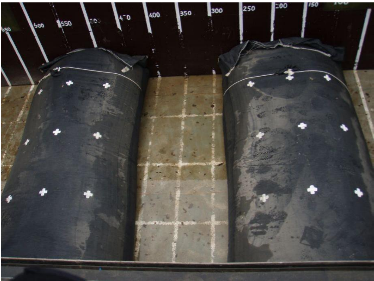
Photo 46: Movement of geotextile tube (left tube) after test series P2-4-2
