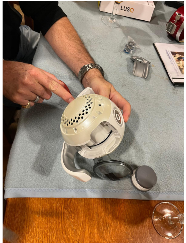
Figure XIII. Realising that there were screws that could open the casing, but hidden under a friction fit ring-shaped cover.
