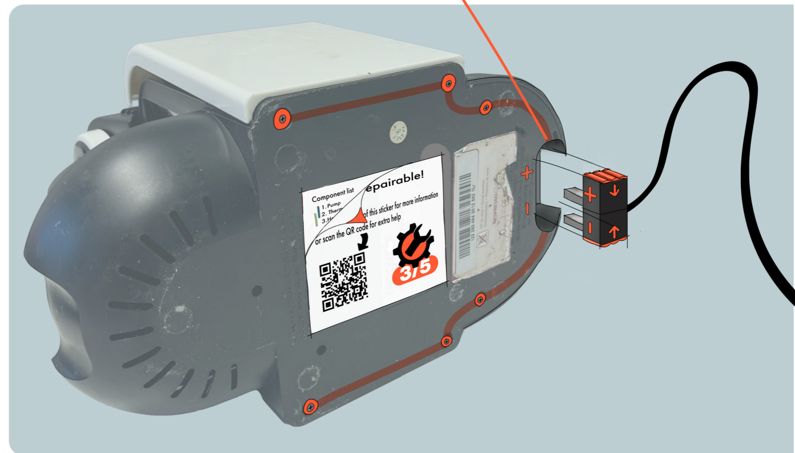
4B The affordance of removing the power source is communicated through physical affordances, such as ridges and an ergonomic casing shape that provides just enough space for finger placement. These features act as physical signifiers, suggesting the intended finger placement. Additionally, symbolic signifiers, such as arrows, reinforce that the user should pinch to disassemble the component.
