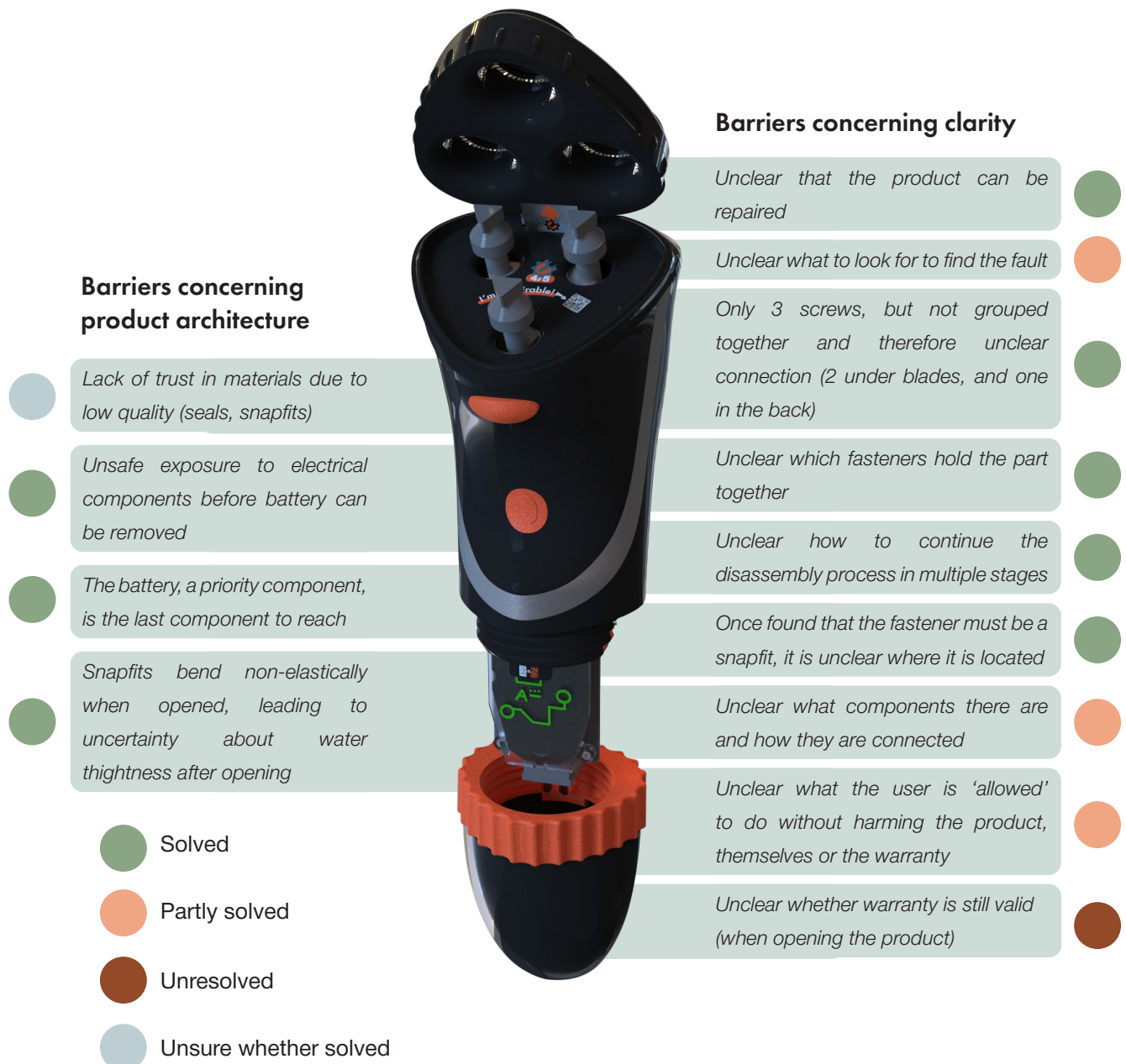
Figure 31. Main barriers accross the DIY repair journey of a Philips shaver, tested against the redesign of the shaver.
