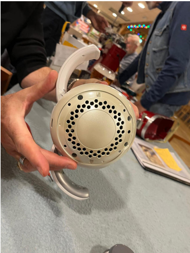
Figure XIII. Realising that there were screws that could open the casing, but hidden under a friction fit ring-shaped cover.
