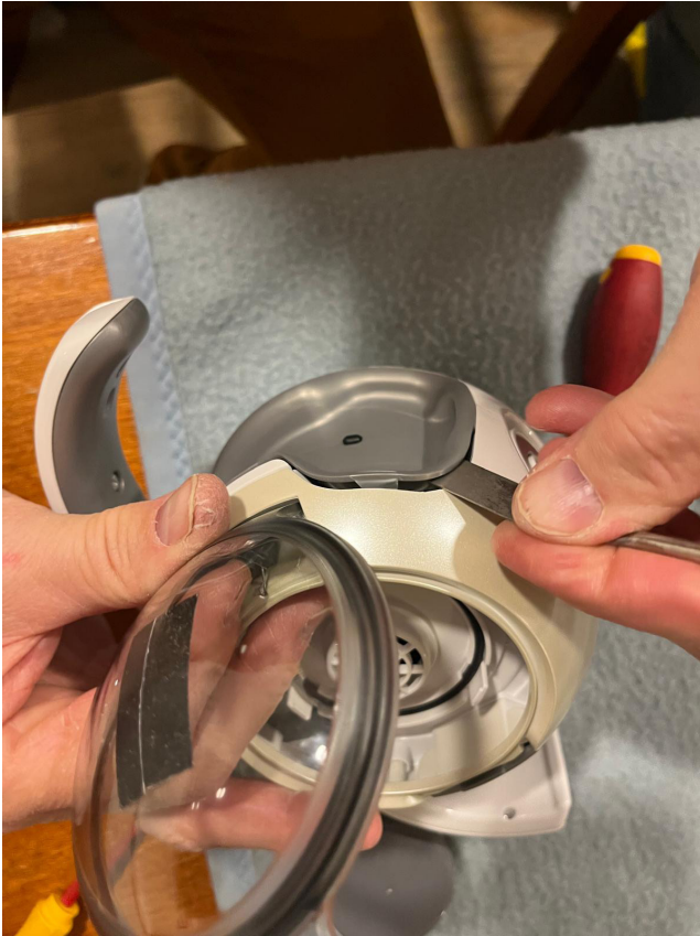
Figure XII. Prying the handheld vacuum open with a spudger and a lot of force.
