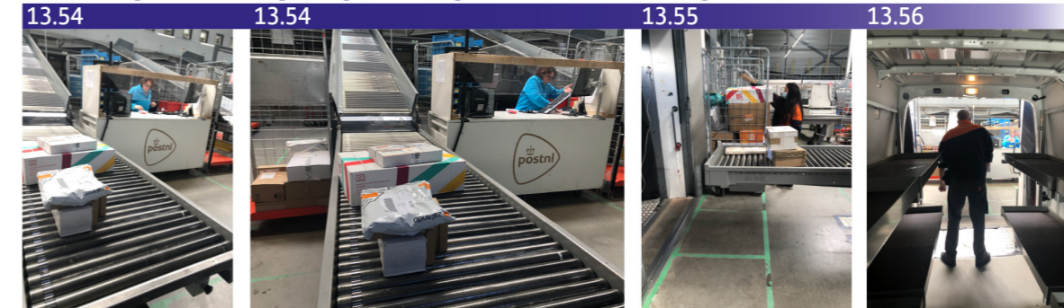
13.54 13.54 13.55 13.56 The packages that need to be sent to a receiver are placed on the rail, waiting to be picked up by runners. The desk clerk checks with the deliverer for irregularities (indicated by the system API such as e.g. unscanned or undelivered parcels). After clarification from the deliverer, this will be solved/notified in the API. Runners are taking the packages (to be send) from the rail, placing them into a trolley. Saying goodbye to the desk clerk and returning the empty delivery van to the parking area.
