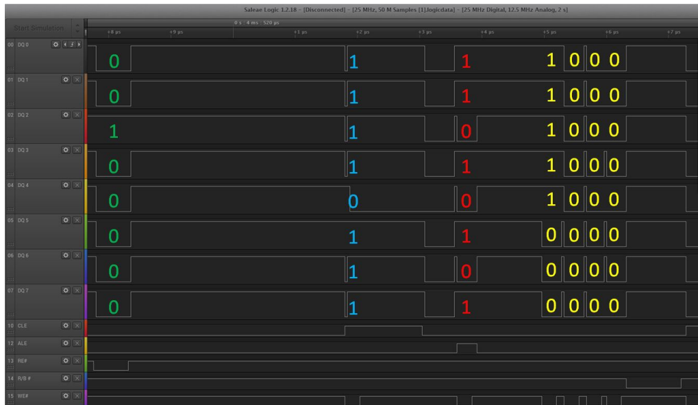
Figure 3.9: Probed signals for setting an offset voltage at index 31
