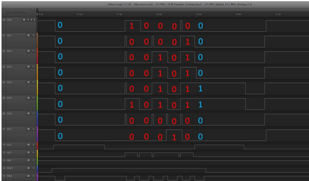
Figure 3.7: Address signals probed by the LogicAnalyzer.
