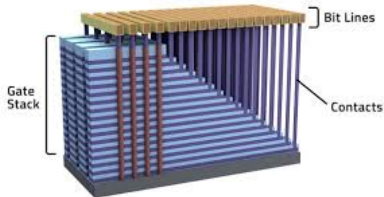
Figure 2.2: Schematic overview of internal 3D NAND memory architecture. [20]
