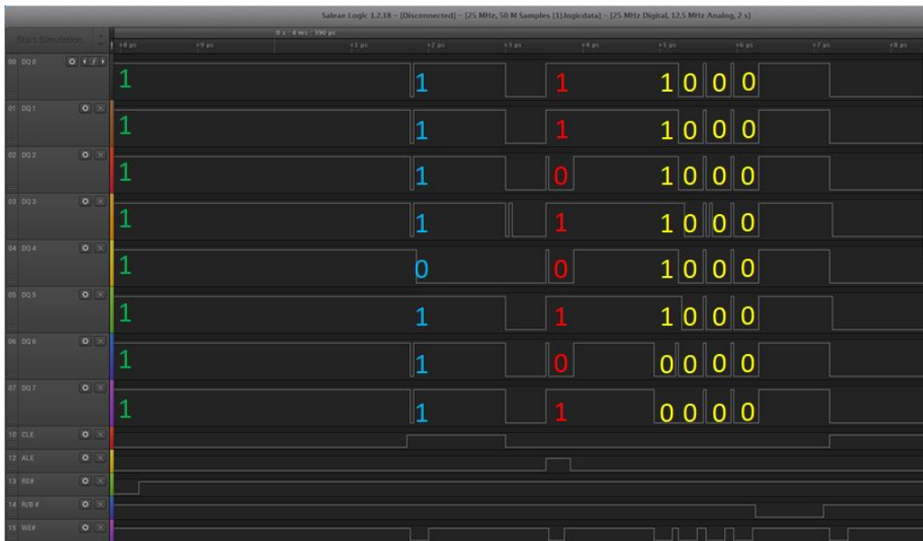
Figure 3.11: Setting the read offset voltage to index 64
