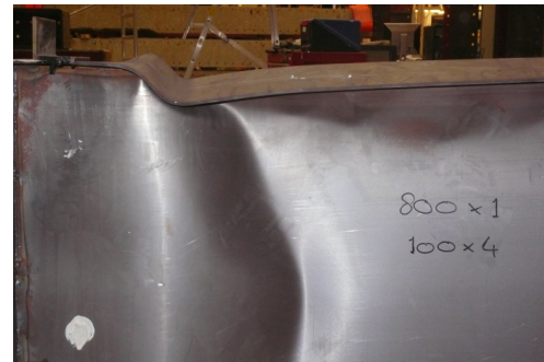
Figure 5-93 Location of the final failure mode of test girder 10, 800x100
