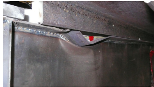
Figure 5-87 Location of the final failure mode of test girder 4, 400x100
