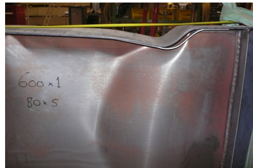
Figure 5-88 Location of the final failure mode of test girder 5, 600x50
