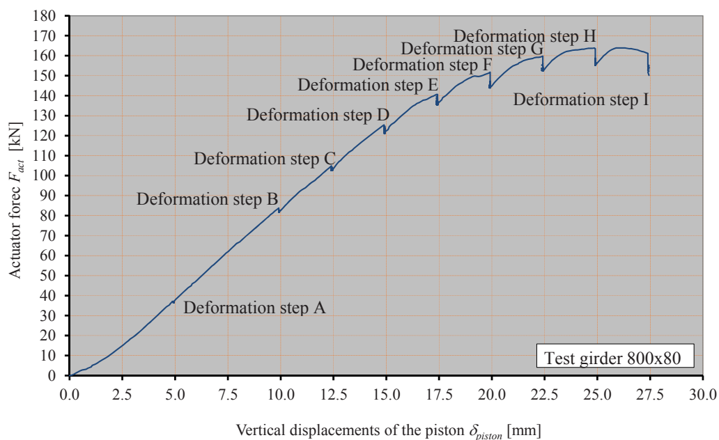
Figure 5-2 The actuator force as a result of the prescribed displacements of the piston for test girder 9, 800x80
