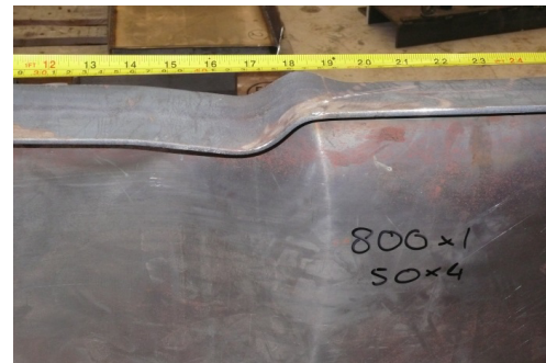
Figure 5-91 Location of the final failure mode of test girder 8, 800x50
