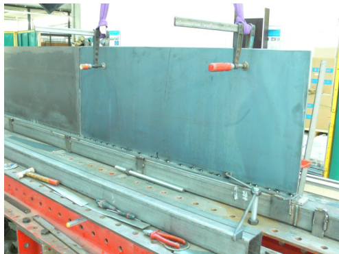
Figure 4-18 Web of the end panel is tag welded to the flange after the web of the test panel
