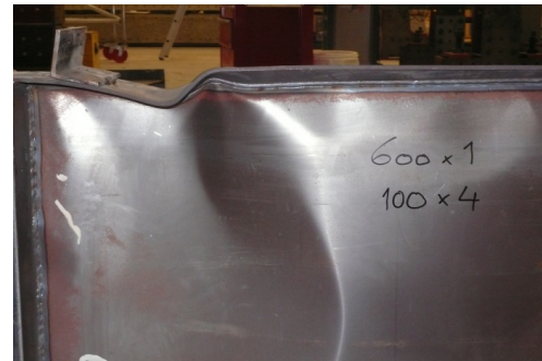
Figure 5-90 Location of the final failure mode of test girder 7, 600x100
