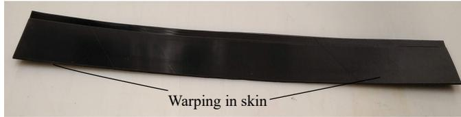
Figure 6.3: Wind tunnel demonstrator skin.
