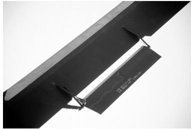
Figure 2.3: Flap used in Kaman helicopters.
