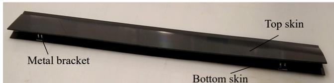
Figure 6.4: Wind tunnel demonstrator flap.
