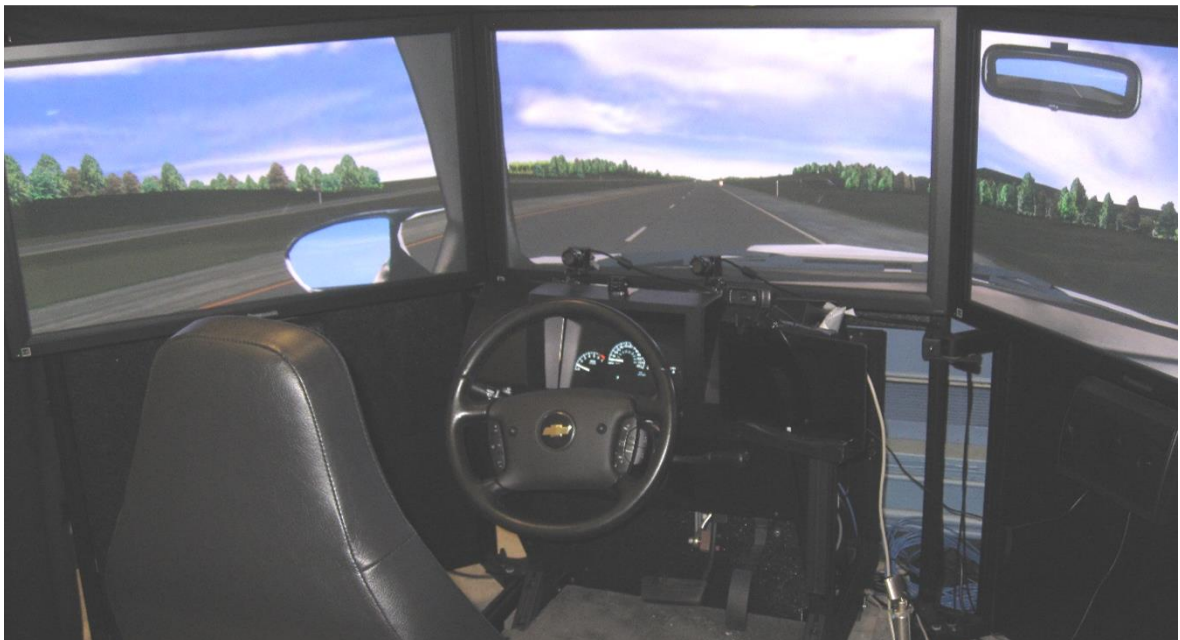
Figure 1. NADS Minisim driving simulator.
