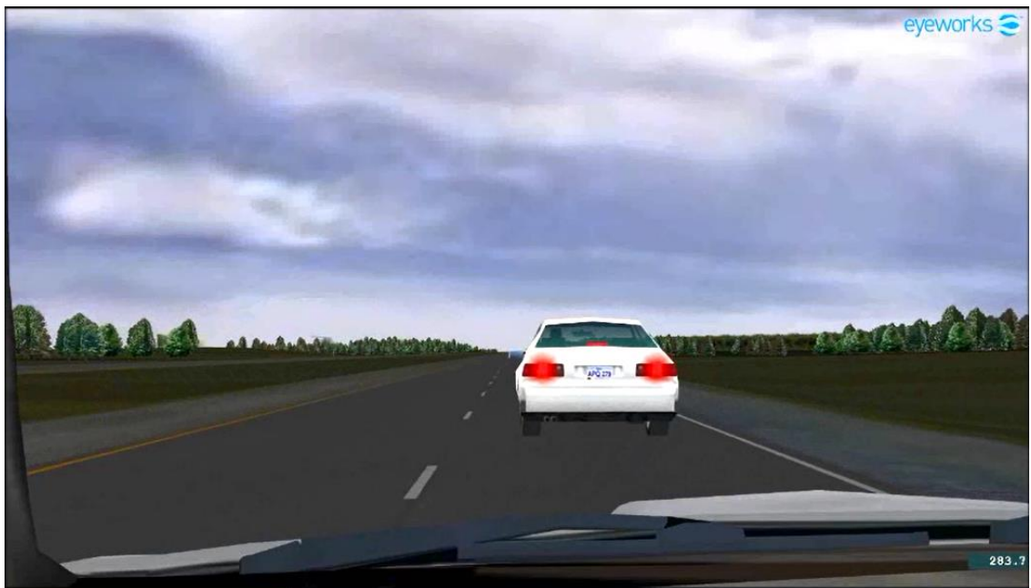
Figure 3. The participant's view of the lead car with brake lights activated. In this view, the bumper-to-bumper distance was approximately 13.4 m.
