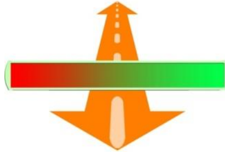
Figure 1. Rear Window Notification Display (RWND): Arrows indicate time headway (THW) deviations (up means that the driver is too far and should close the gap; down means that the driver is too close and should open the gap) and the horizontal bar indicates lead vehicle acceleration (right, color coded with green is acceleration; left, color coded with red is deceleration).
