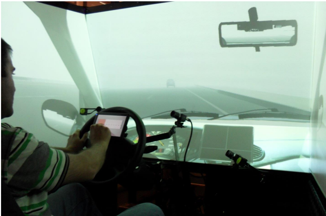
Figure 1. Driving simulator in the experimental setup. The lead car is driving 31 m ahead of the participant's car. The driver is indicating the level of risk he is feeling on the touchscreen mounted on the steering wheel. Note that the eye-tracking equipment was not used in this experiment.
