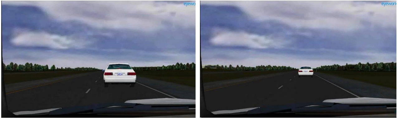
Figure 5. The participant's view of the lead car when the bumper-to-bumper distance was approximately 13.4 m (left) and 33.4 m (right).
