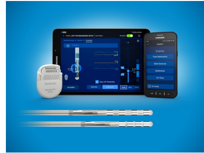
Figure 5: Image showing the Percept IPG (left) the Percept Clinician Programmer Tablet (middle), a Patient Programmer on the phone to track events (right) and an example of implanted electrode leads with various contact electrode points. Image taken from [27].
