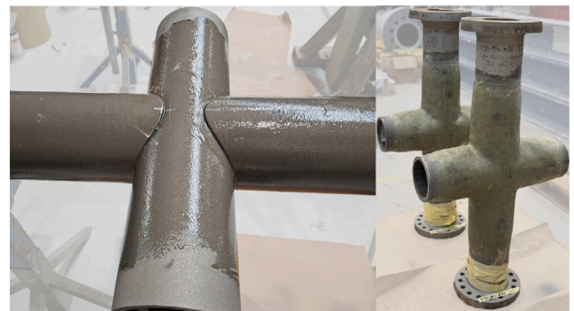
Fig. 3. X90 joint during manufacturing: before lamination (left) and after composite lamination (right).
