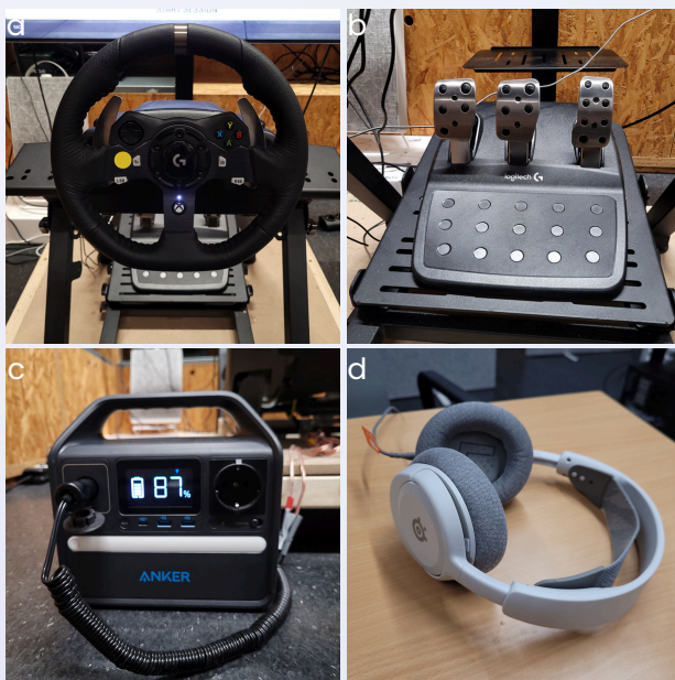
Fig 10: (a) A close up of the steering wheel. Notice the yellow traction control sticker (b) The three pedal setup of the simulator – rightmost accelerator, middle brake (c) Portable power supply for the electronically adjustable driver seat (d) Headphones used for the stressor – wired but lightweight and unintrusive
