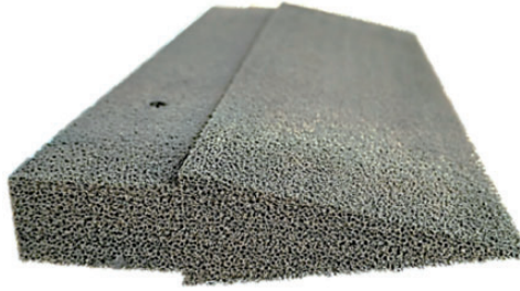
Figure 4. Metal foam trailing-edge insert used in the experiment. The total length of the insert is 0.06 m. Extracted from Carpio et al. 41
