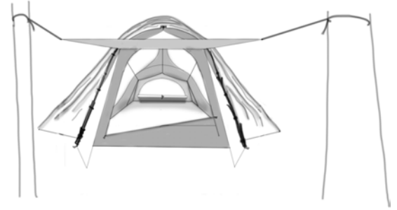
Or replace two third of the front tent pole by two trekking poles
