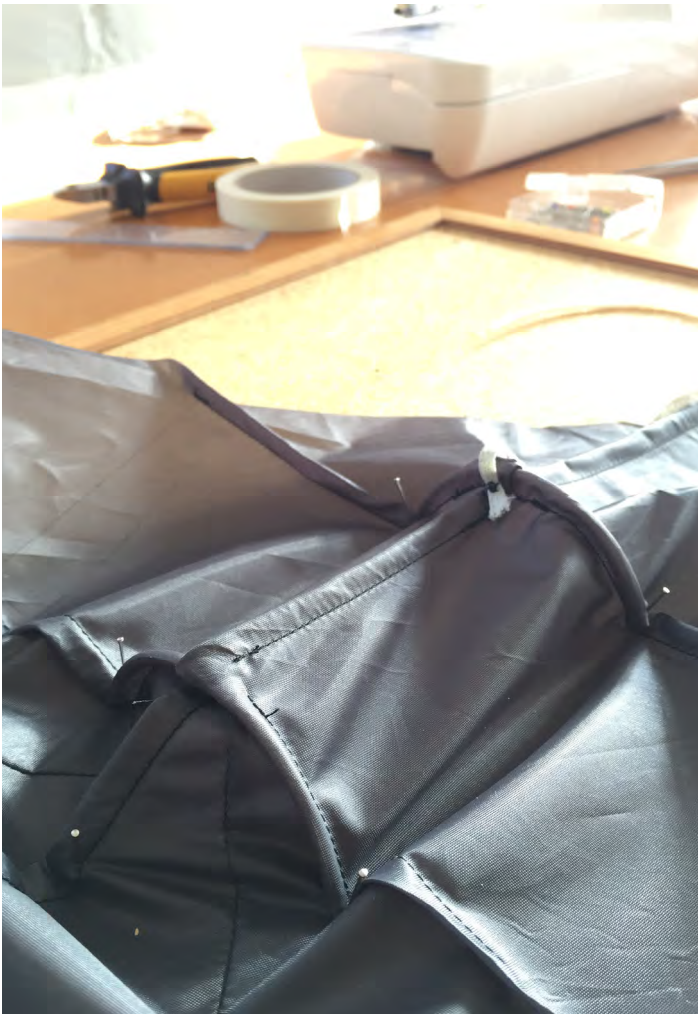
Figure 90. Study how one piece of fabric fits different pole structures
