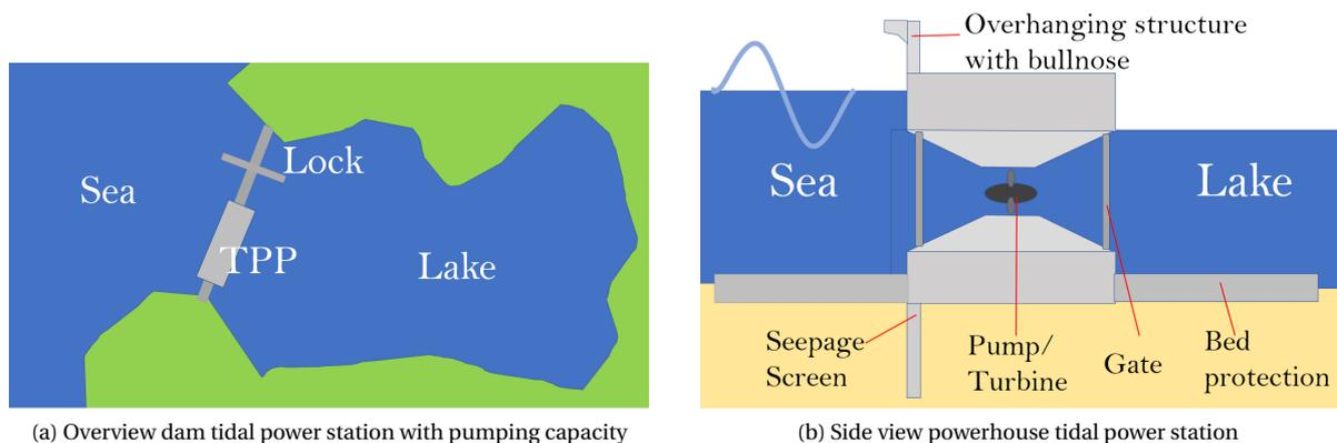
Figure 1: Dam with tidal powerstation with pumping capacity
