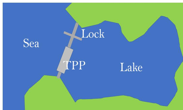
Figure 4.1: Overview conceptual design Dam with tidal power plant
