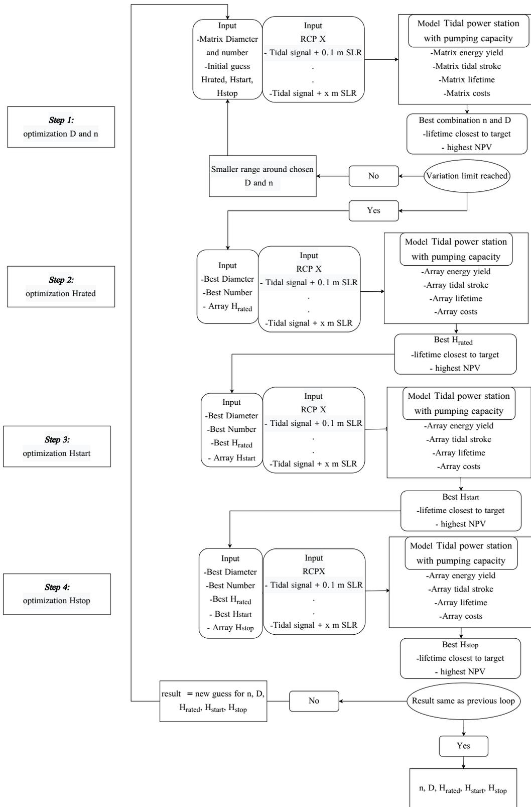
Figure 6.5: Workflow computer model optimisation
