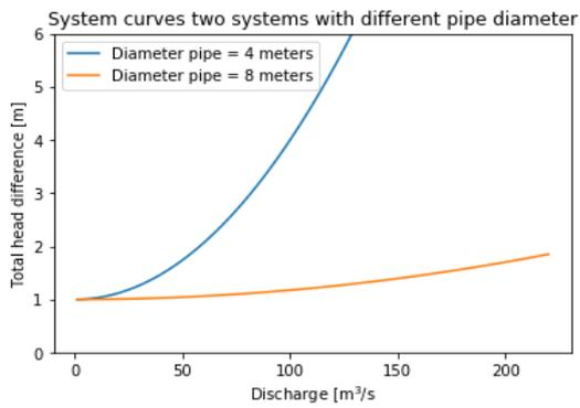
(c) System curves for system with different pipe diameters, static head = 1 meter
