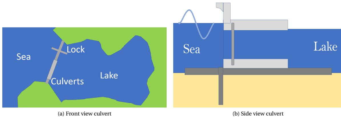
Figure 8.2: Conceptual design culverts
