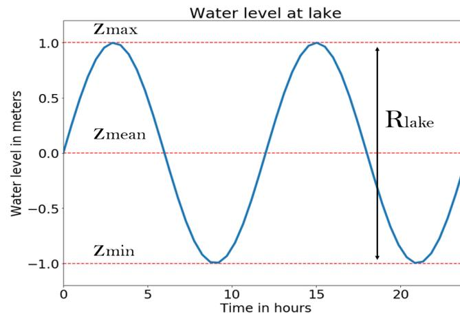
Figure 2.1: Minimum, mean and maximum water level and the tidal stroke at a lake
