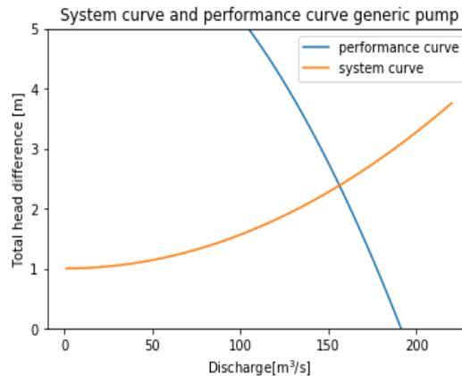
Figure 5.7: System and performance curve for generic system and pump
