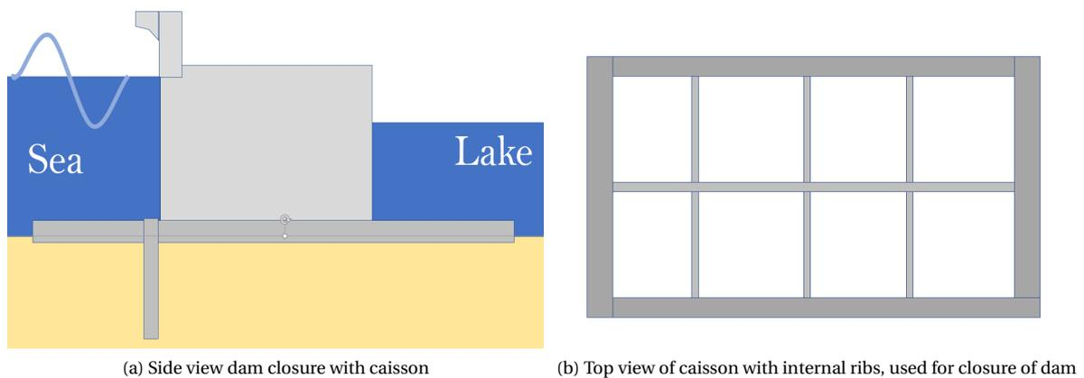
Figure 4.3: Conceptual design closure dam
