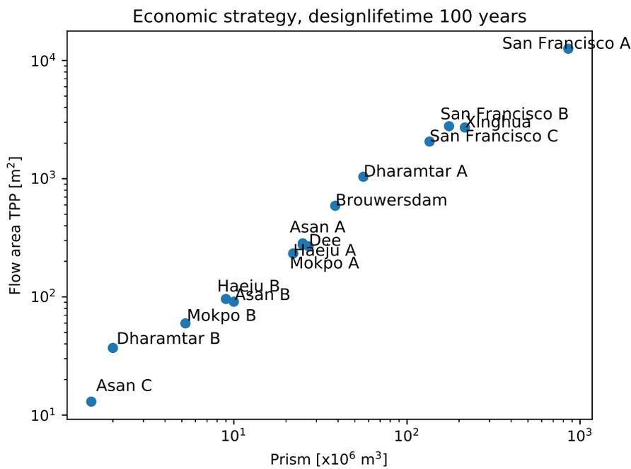
Figure 7.4: Prism versus flow area
