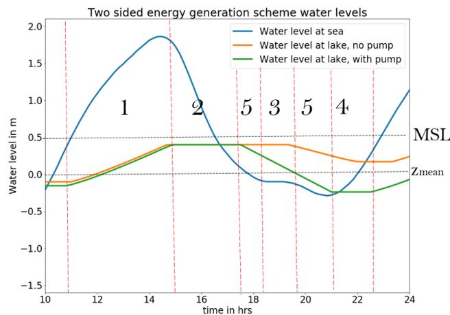
Figure 5.4: Two sided energy generation scheme, with pump
