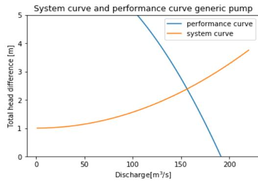
(d) System and performance curve for generic system and pump
