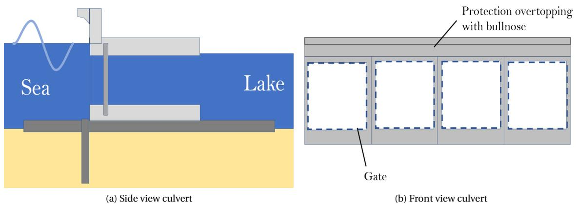
Figure 4.5: Conceptual design culverts
