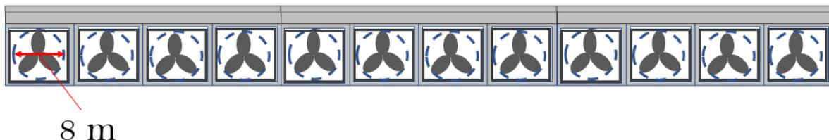
Figure 5.8: Design Brouwersdam: 12 pump/turbines with 8 meters diameter
