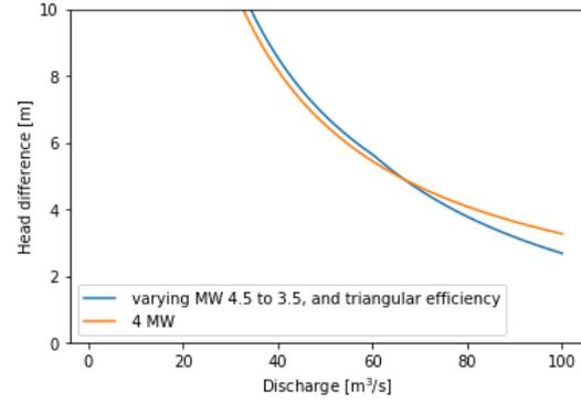
(b) Performance curve based on capacity with effect for power and efficiency included
