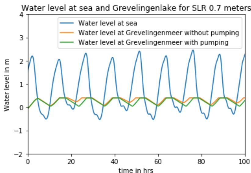
Figure 1.2: Illustration functioning pumping system to regulate water level at Grevelingenlake
