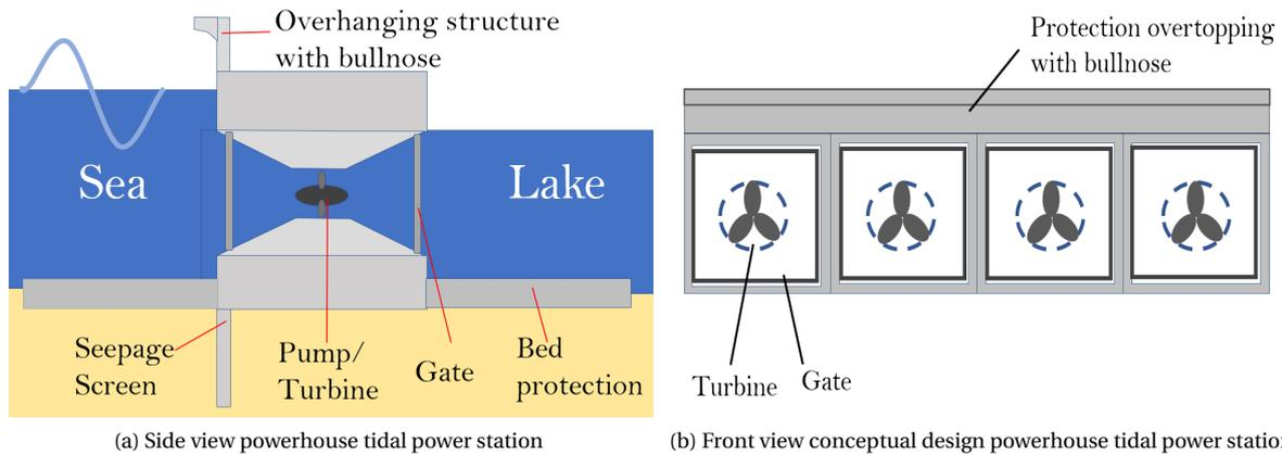
Figure 4.2: Conceptual design powerhouse
