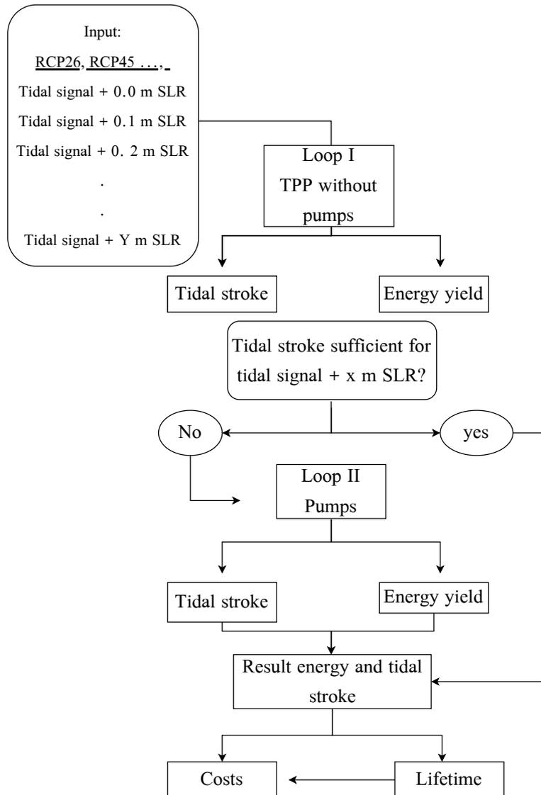
Figure 5.5: Workflow computer model
