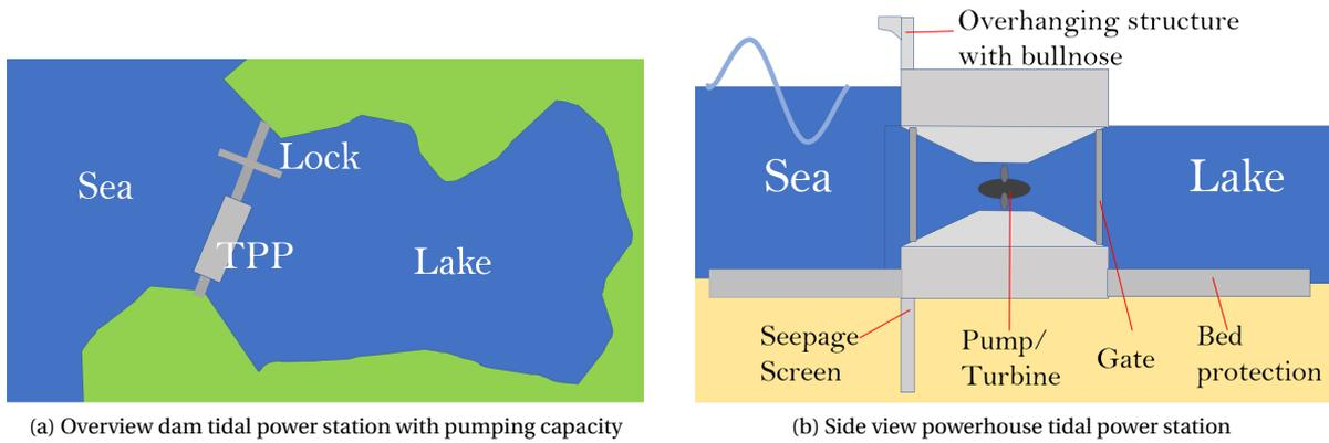
Figure 8.1: Dam with tidal powerstation with pumping capacity
