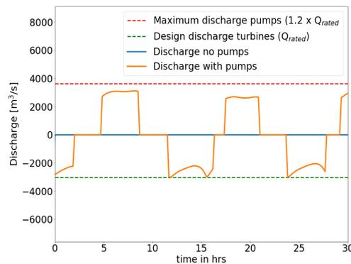
(f) Discharge through pump/turbines at 1 meter sea level rise
