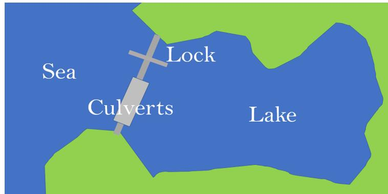
Figure 4.4: Overview conceptual design Dam with culverts
