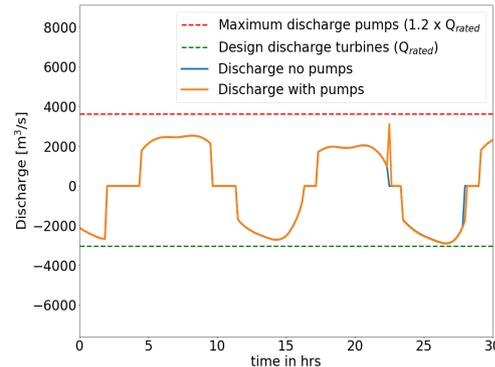
(b) Discharge through pump/turbines at 0 meter sea level rise
