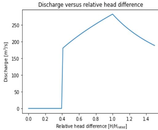
Figure 5.6: Discharge versus relative head, maximum is at  $H/H_{\text{rated}} = 1$
